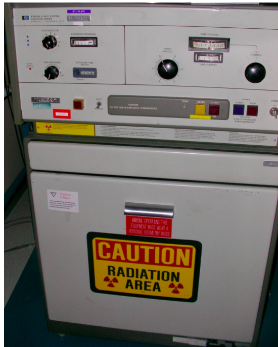
Figure 54: X-ray System used to test Selenium-CMOS PPS array
