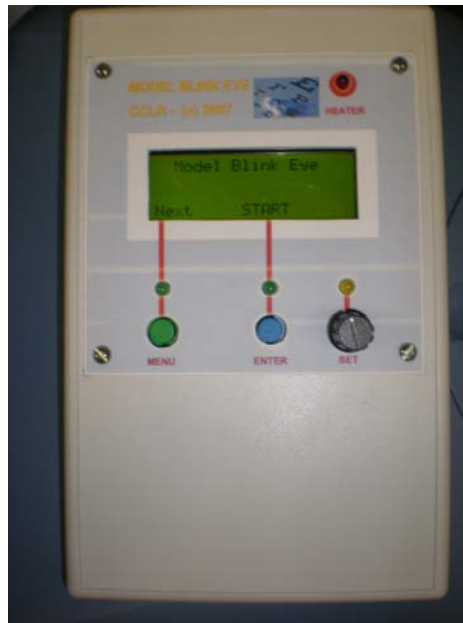
Figure 5-2: Control box which controls temperature, purge and refill times, and amount of time lenses in and out of the fluid bath.
