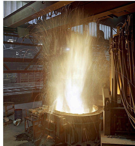
Fig.2.33 An electric arc furnace melting steel scrap
