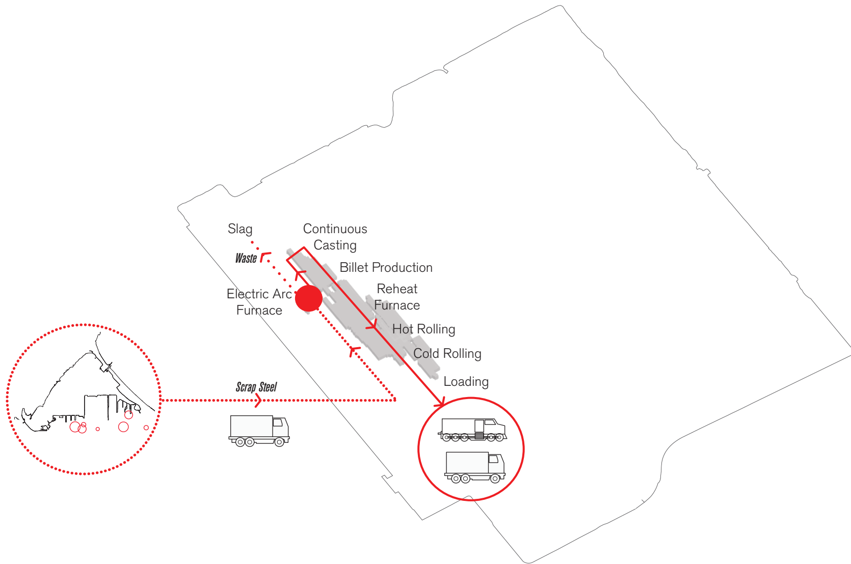
Fig.2.31 Operations of a typical steel mini mill, and their relative scale on the site
