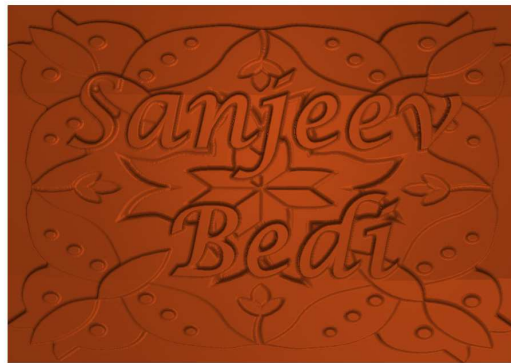
(b) Simulation of finishing pass using ball nose cutter, r_1 = 1.5875mm and r_2 = 0.0mm
