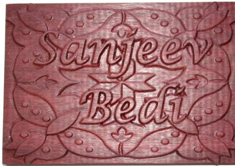
(c) Machined plaque, r_1 = 1.5875mm and r_2 = 0.0mm
