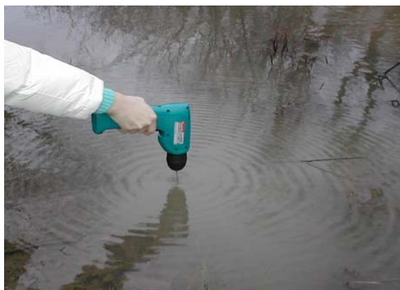
Figure 3-3 On-site sampling of river water using the thin film sampler.
