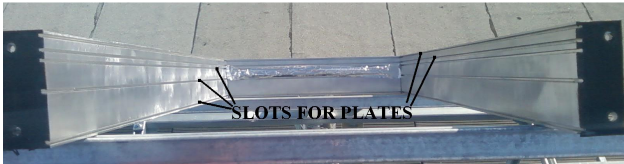
FIGURE 4.5 OPENED COLLECTOR SHOWING THE SLOTS IN WHICH THE PLATES ARE INSTALLED
