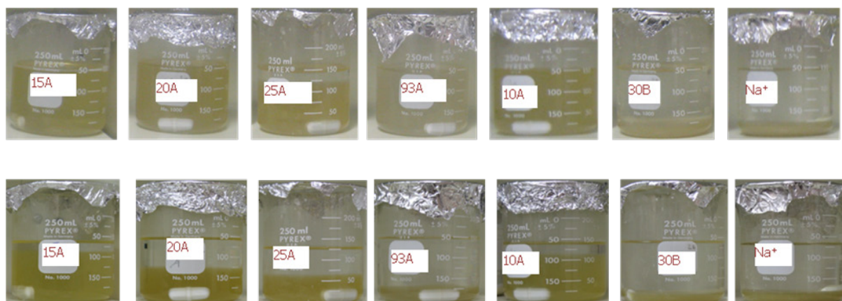
Figure 4.2. Comparison between the sedimentation of different Cloisite samples in toluene at room temperature, after one day (top) and after two weeks (bottom).
