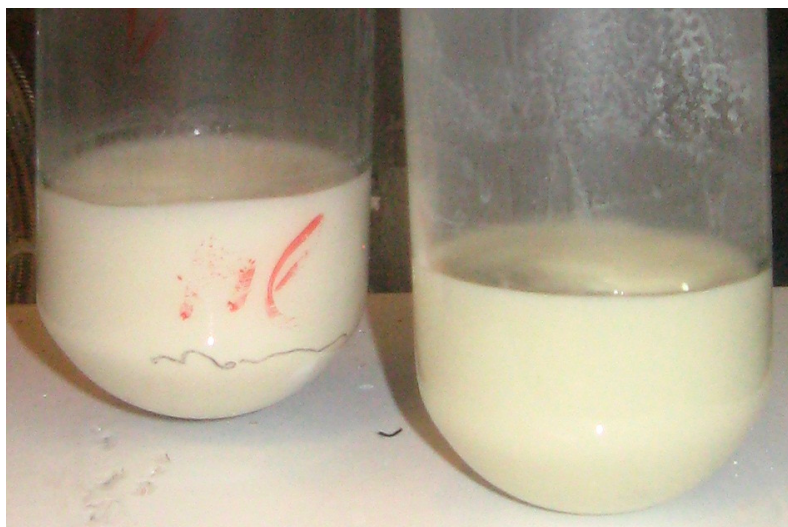
Figure 6.1. Dispersion of Cloisite 93A in toluene (right) and hexane (left) (the picture was taken during stirring).
