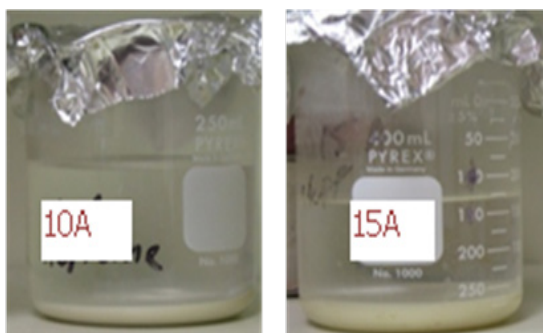
Figure 4.3. Sedimentation of Cloisites 10A and 15A in heptane after one day.
