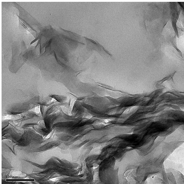
Figure 5.24. TEM image of B10 particles embedded in epoxy resin for ultra-microtome.
