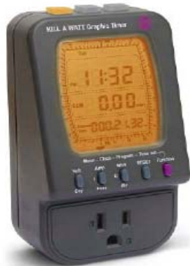
Digital Programmable Timer to simulate the EHMS ON/OFF decisions
