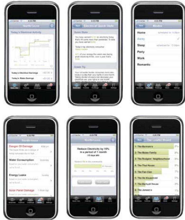
Figure 3.6 The iPhone application allows ubiquitous access to full home monitoring and control.
