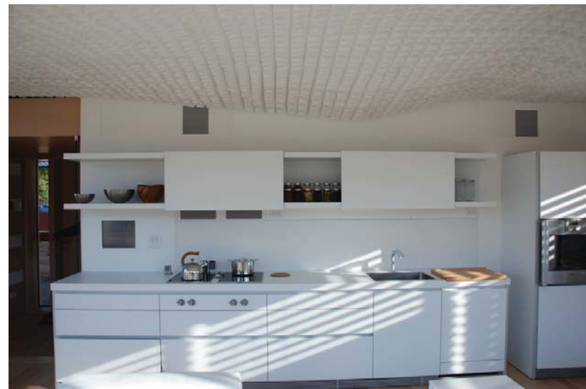
Figure 2.32: Lighting condition in Kitchen when exterior shades on east facade are in solar block mode with clerestory tilt zone open.
