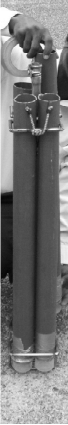
Figure 3-2 Sediment trap sampler constructed of four PVC tubes secured in a metal frame by bungee cords and fitted with sampling cups at the base for sediment recovery. A drainage spout at 5 inches from the cups was drilled and sealed with duct tape until retrieval.
