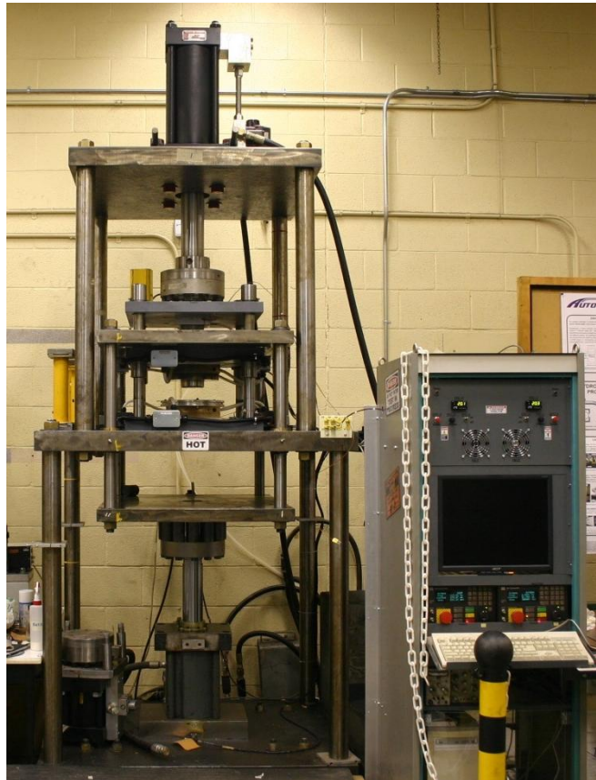
Figure 3.3: Servo-hydraulic press at the University of Waterloo.
