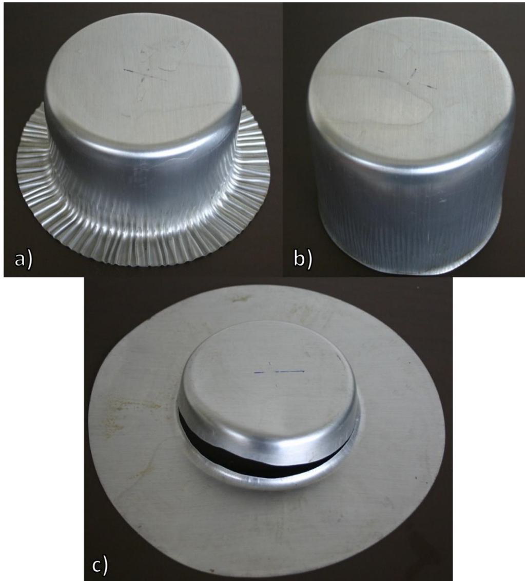
Figure 5.11: Nine inch diameter blanks drawn at 300°C showing a) wrinkling, b) complete draw, c) failure.
