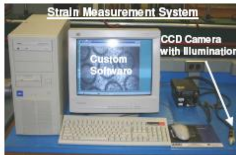
Figure 3.6: Strain measurement system
