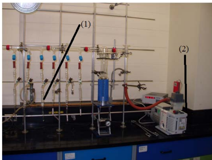
Figure 2.14 An evacuation system with (1) silica tubes connected to the vacuum line; (2) a rotary pump providing the vacuum.
