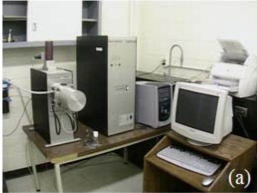
Figure 2.24 (a) The FlashLine 3000 device; (b) the sample holder.
