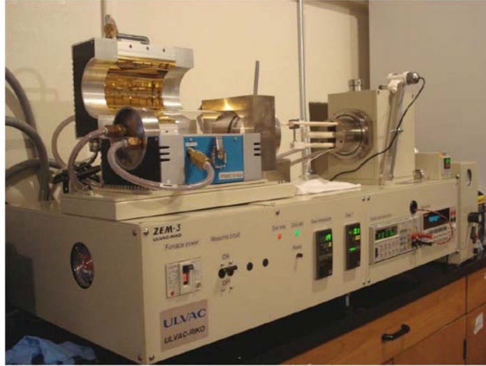
Figure 2.21 ULVAC ZEM-3 Seebeck coefficient/electrical resistance measuring system 54 .
