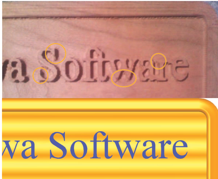
Figure 2.5: Comparison of actual machined sign with 3D CAD model
