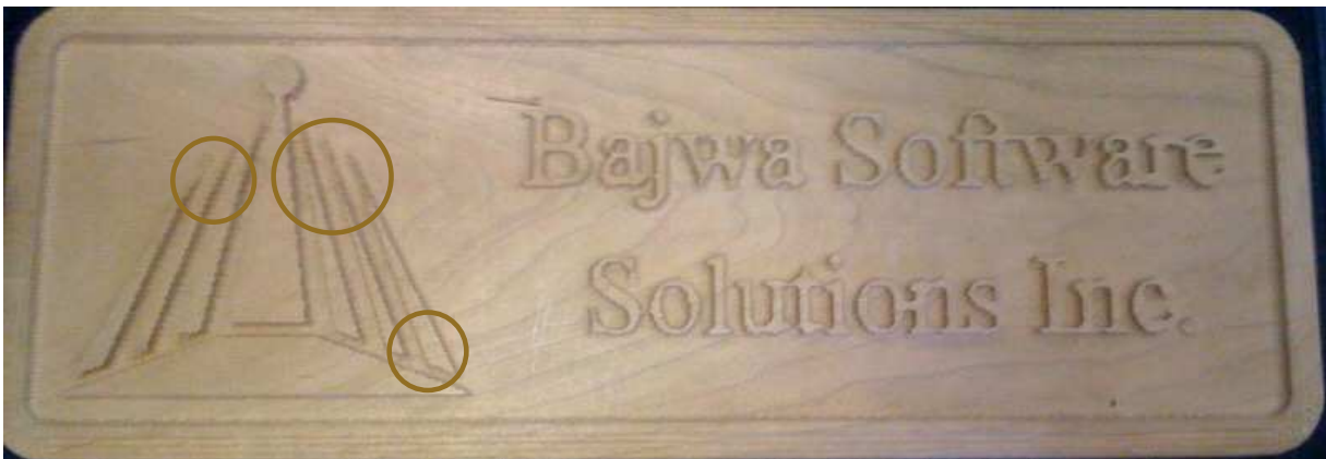
Figure 2.4: Machining results of wooden sign using Ball-Drop method
