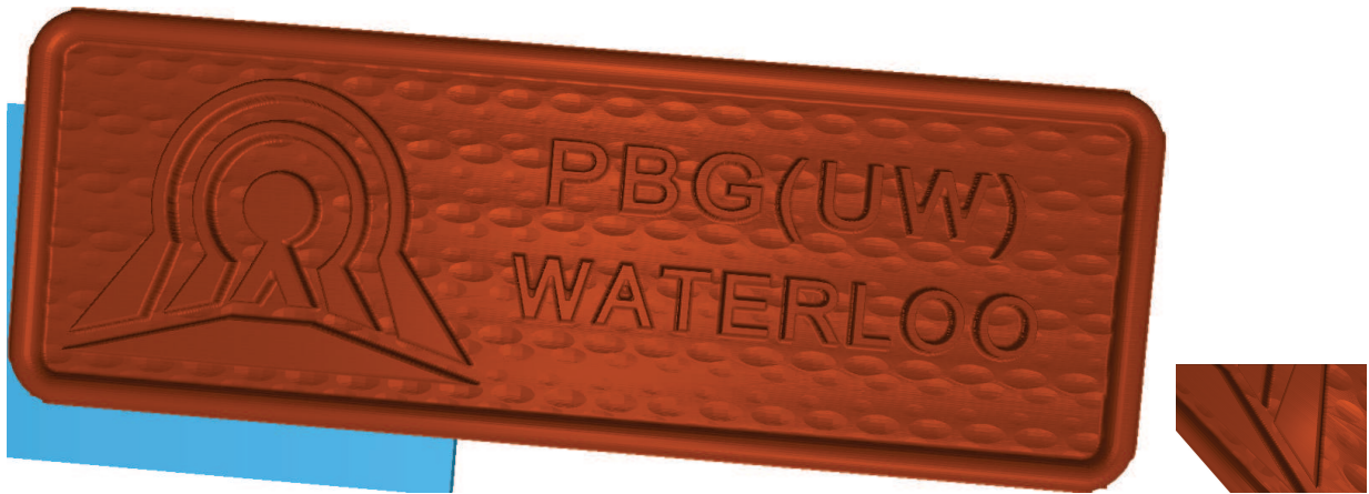
Figure 4.8: Simulation Results on ToolSim using ball nose end mill
