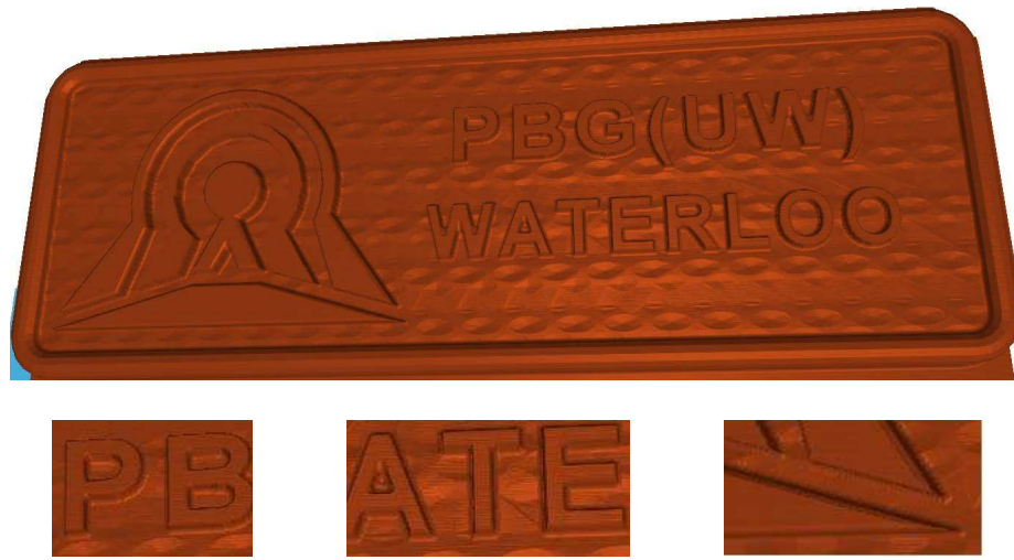
Figure 4.15: Tool path Generated after applying pencil tool path
