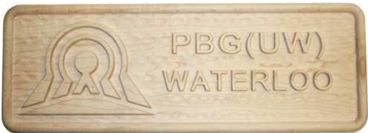
Figure 4.16: Wooden sign machined in 3 axis CNC milling machine
