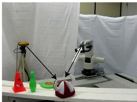
Figure 6.13: Experiment 4: The manipulator points to the object on which the camera focuses
