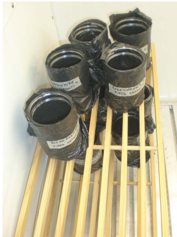
Figure 5.1: Incubation jars and configuration within the environmental chamber for the CO 2 treatment after t=6 destructive sampling.
