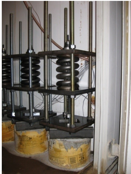
Figure 3.5 – Creep test setup (2) inside the environmental chamber for freeze/thaw exposure
