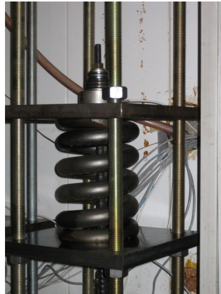
Figure 3.5 – Creep test setup (2) inside the environmental chamber for freeze/thaw exposure
