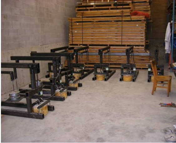
Figure 3.4 – Creep testing setup (1) for room temperature and moisture exposure
