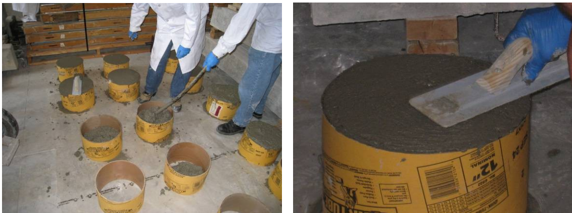
(a) Specimen concrete pouring
