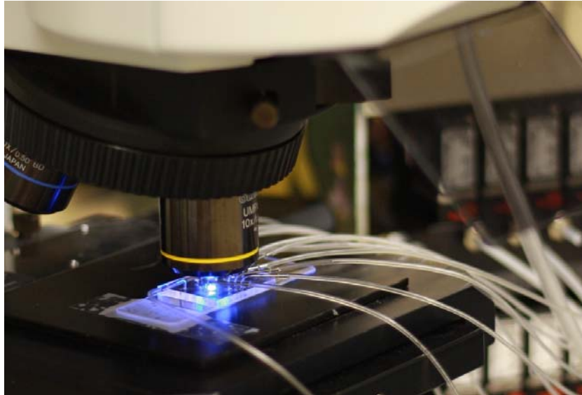
Figure 3 Image-based Microflow Cytometer with Integrated Pumps and Valves
