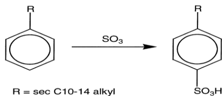
Figure 2.4 Sulfonation of Linear Alkylbenzene to produce Linear Alkylbenzene Sulfonic Acid
