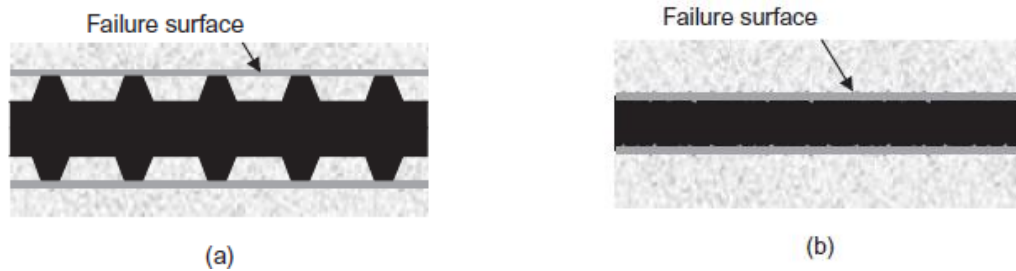
Figure 3: Failure surface in the case of pull-out failure of (a) a ribbed bar and (b) a smooth bar (K. Lundgren, 2007)
