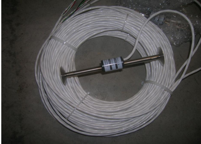
Figure 35 Vibrating Wire Asphalt Strain Gauge
