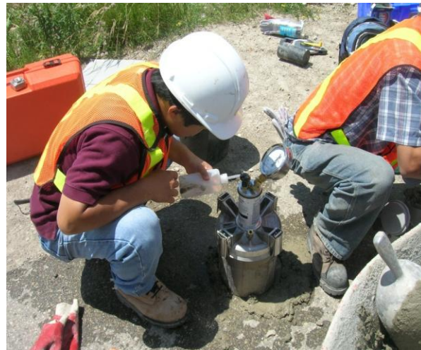
Figure 43 On-site Concrete Air-Void Testing
