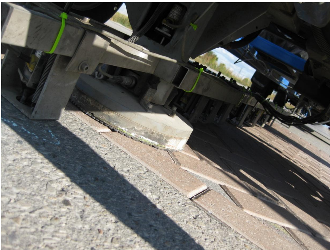
Figure 112 FWD Testing on SSGBAH
