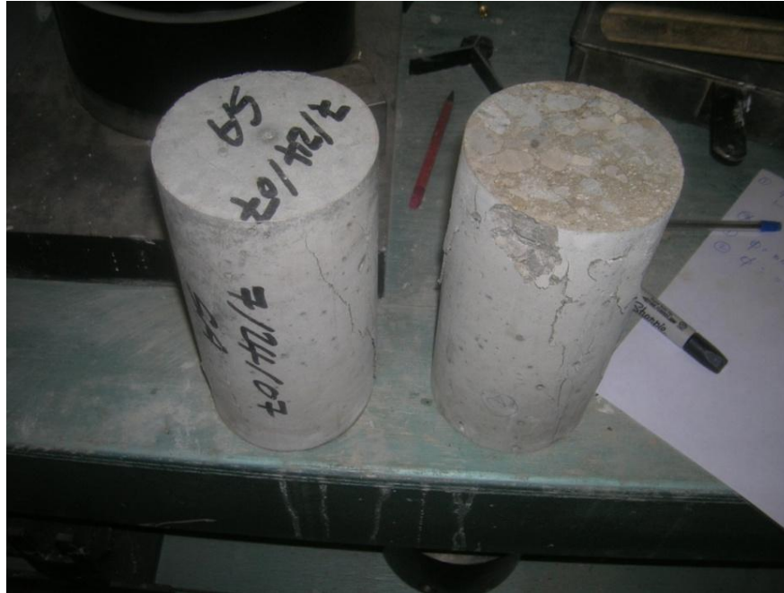
Figure 74 A Cylinder After Compressive Strength Testing
