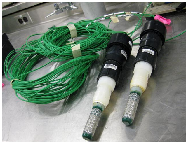
Figure 28 Moisture Sensors Ready to Install in SSGBAH
