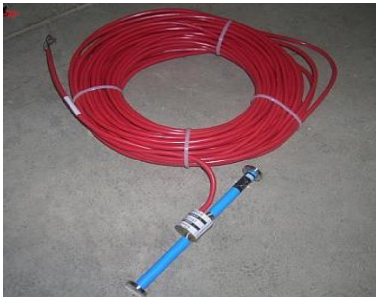
Figure 36 Vibrating Wire Concrete Strain Gauge
