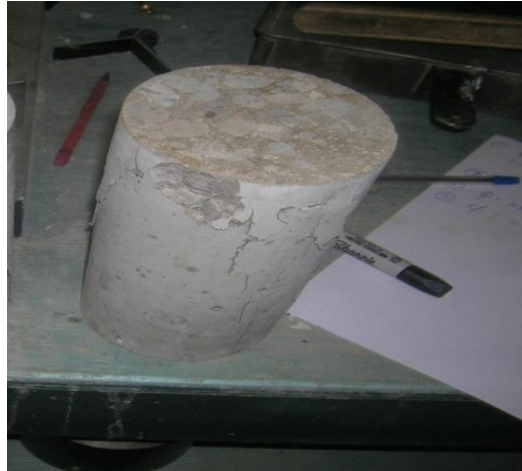
Figure 45 A Cylinder after Compressive Strength Testing
