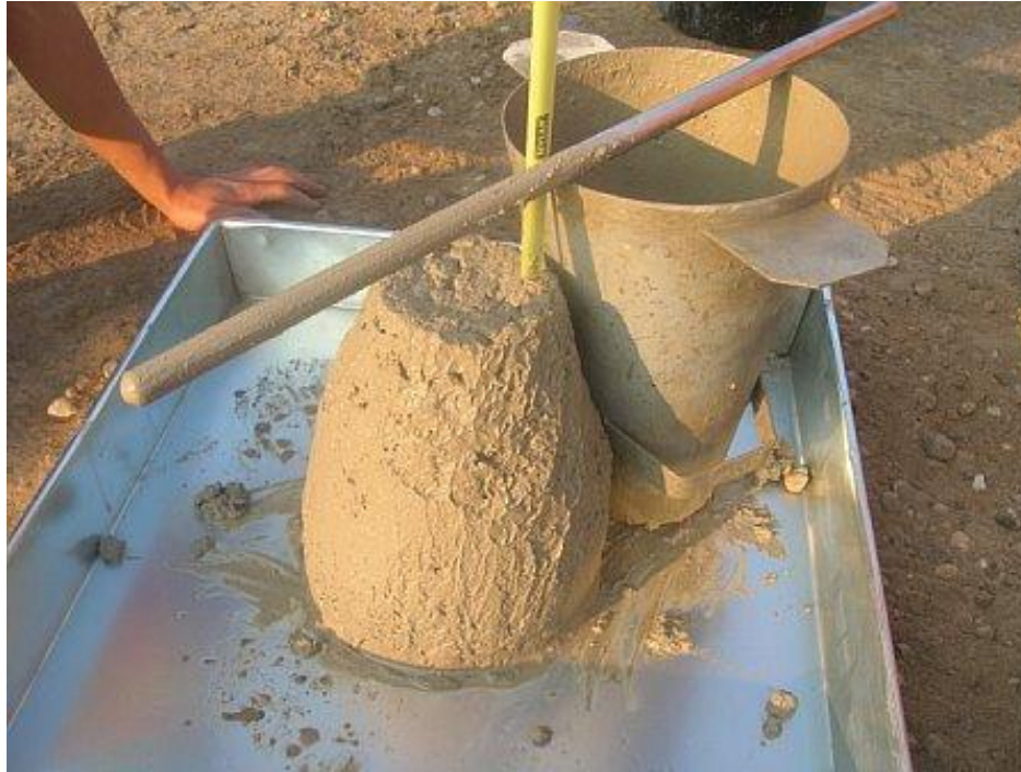
Figure 73 On-site Concrete Slump Testing
