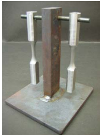
Figure 4.11: Apparatus used to hang specimens during annealing process
