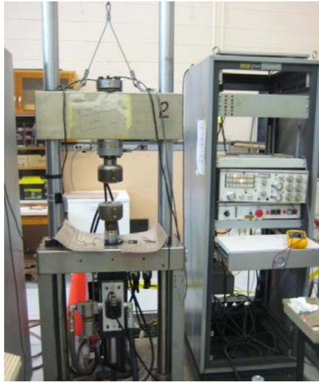
Figure 4.10: Cyclic test frame using MTS 442 controller
