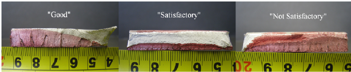
Figure 4.6: Dye penetrant quality classification
