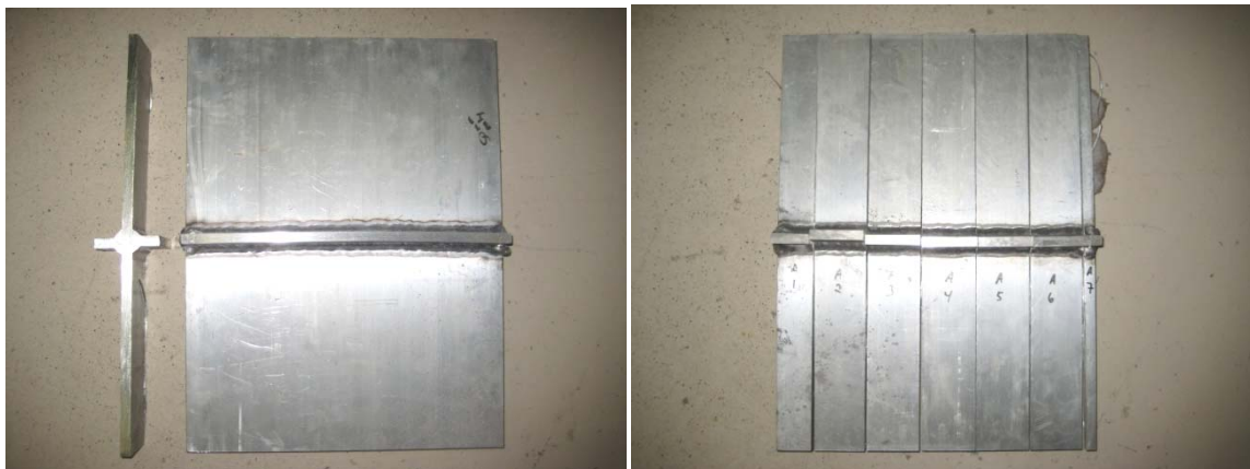
Figure 4.3: Specimen fabrication; aluminum panels (left) and saw-cut specimens (right)
