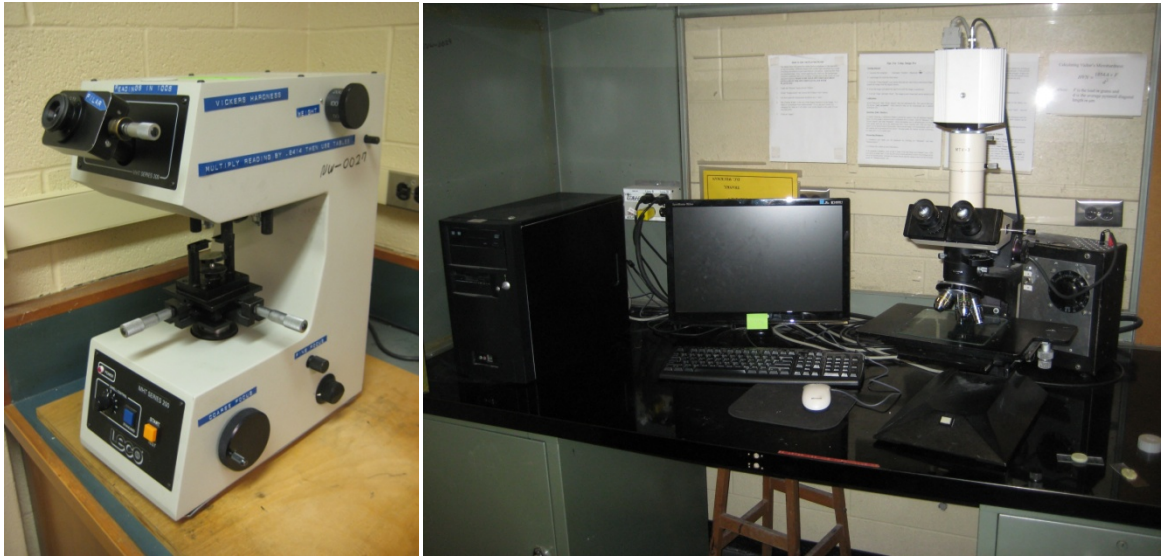
Figure 4.16: Vickers hardness machine (left) and high-powered microscope (right)
