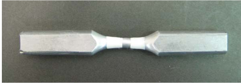
Figure 4.12: Cyclic test specimen with M-Coat
