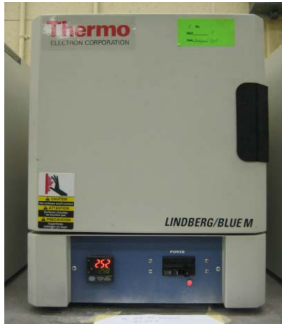
Figure 4.8: Oven used for full annealing of aluminum specimens
