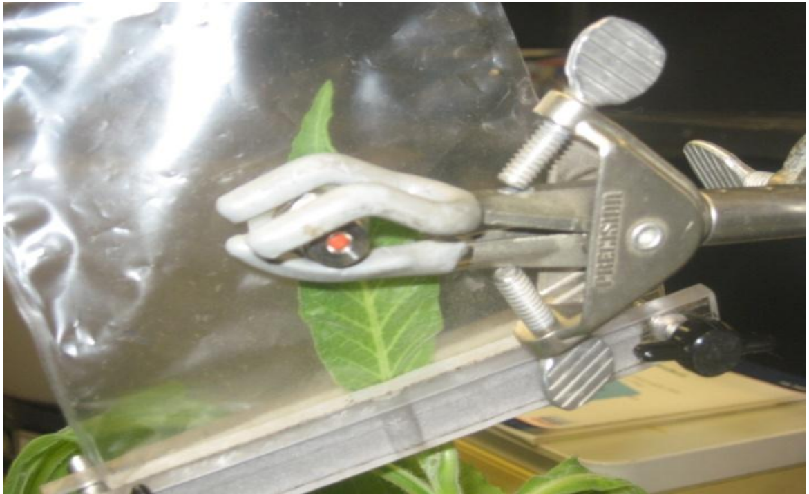
Figure 1: A young tobacco leaf is enclosed in a Tedlar bag and the open end of the bag is closed with a clamp.
