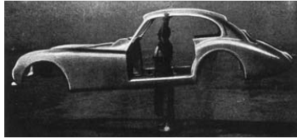
Figure 1.2: Car body developed by Allard in 1952 and made of magnesium sheet [10]
