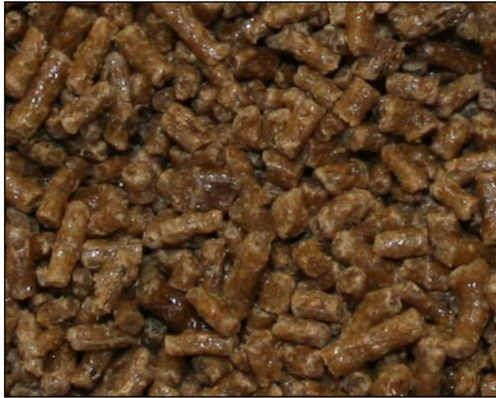
Figure 3-5: Granulated composite of Nylon-6/ wheat straw filler 15 wt- %
