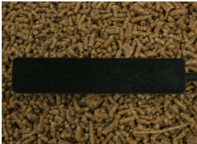
Figure 4-1: Nylon-6 with 15 wt-% of wheat straw: extruded pellets and innjection moulded test bar
