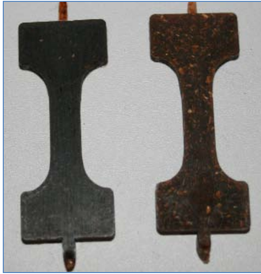
Figure 4-2: Comparison between color of sample with 4 wt-% salt(left) and sample with 4 wt-% of plasticizer(right)
