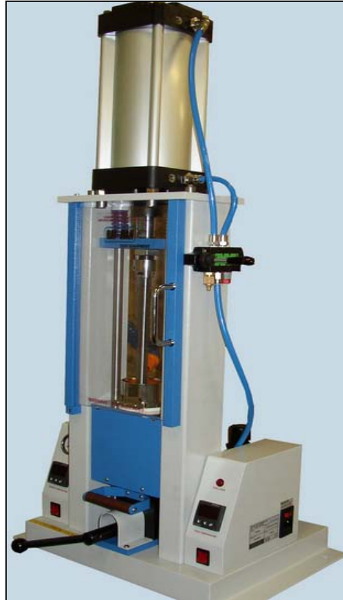
Figure 3-6: Lab scale Ray Ran injection moulding
