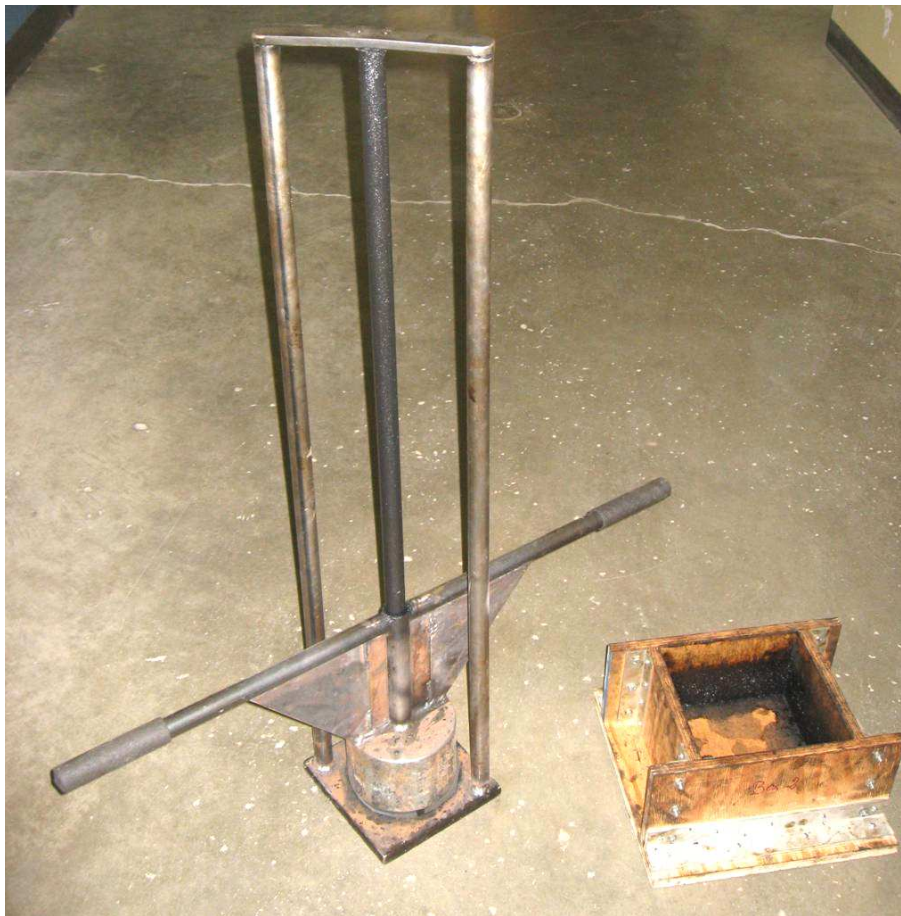
Figure 6-2: Hand hammer and mould used for compaction of HMA slab specimens
