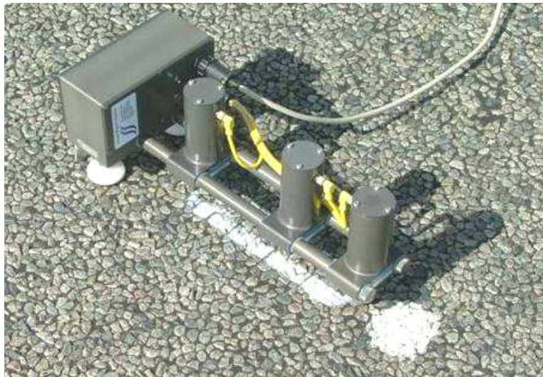
Figure 4-14: Portable seismic pavement analyzer (Steyn and Sadzik 2007)
