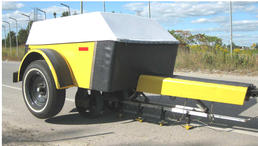
Figure 4-4: Dynaflect in the test position
