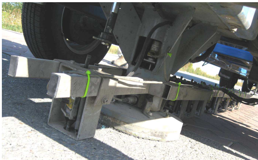
Figure 4-5: Dynatest FWD in the test position
