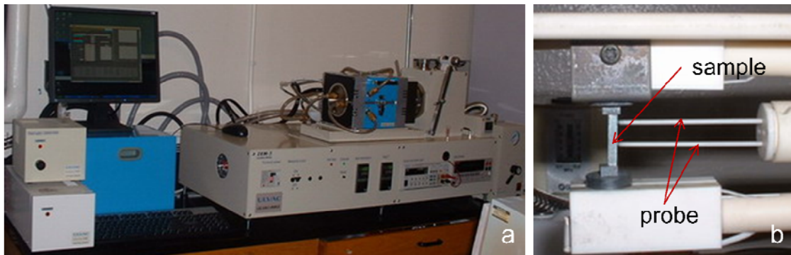
Fig. 2.15 (a) ULVAC ZEM-3 measuring system; (b) the sample placed between the electrodes with two probes contacts.
