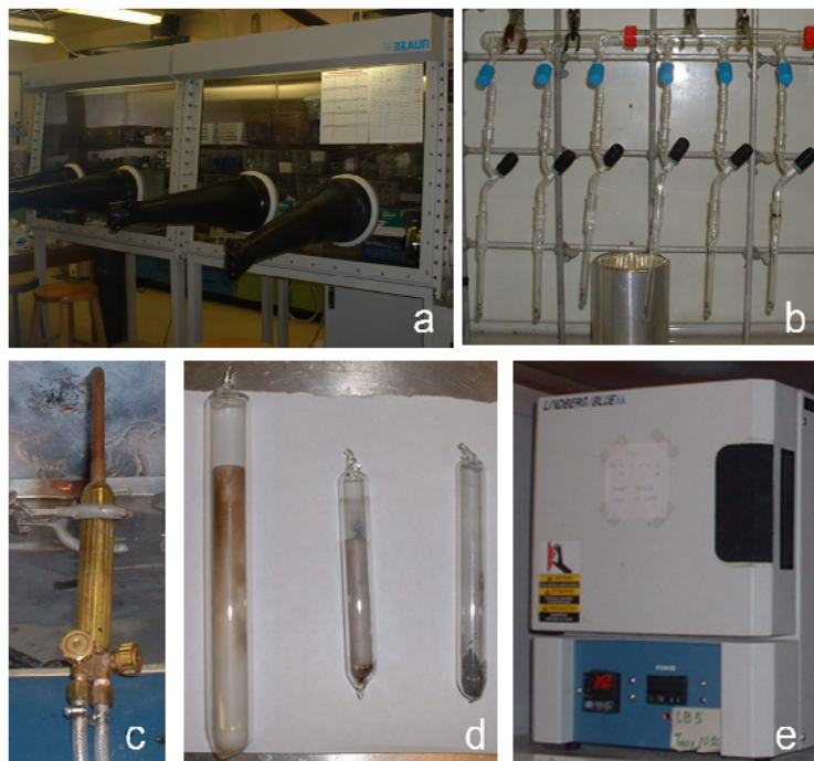
Fig. 2.2 Steps for sample preparation. (a) glove box; (b) vacuum line; (c) H 2 /O 2 torch; (d) sealed tubes; (e) resistance furnace.
