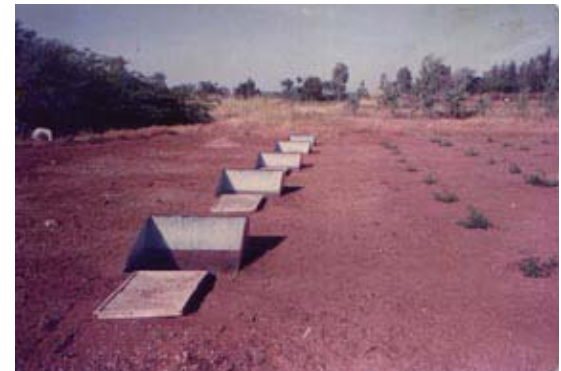
fig. 3.18 Experimental solar stills in India
