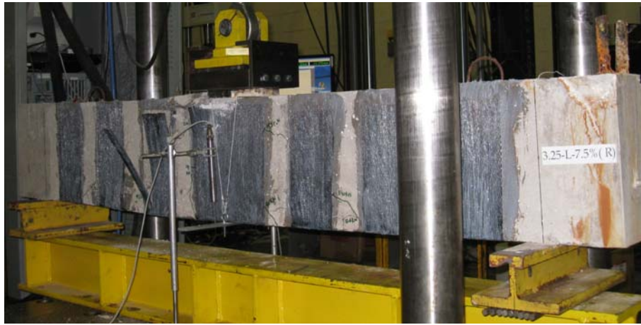
Figure 4.30: Failure mode of FRP repaired corroded beam (3.25-L-7.5%- R)
