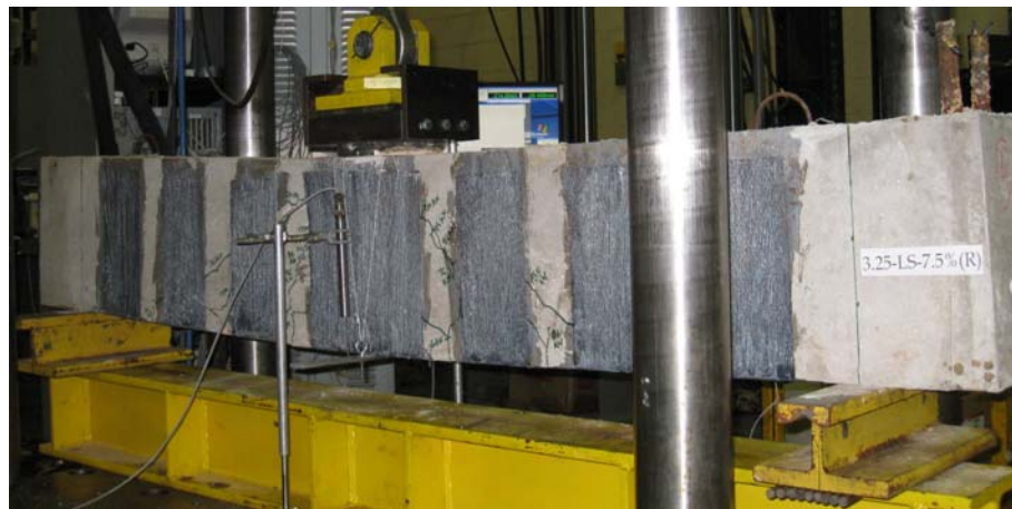
Figure 4.43: Failure mode of FRP repaired corroded beam (3.25-LS-7.5%-R)
