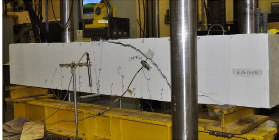
Figure 4.32: Failure mode of control beam 1 (series B-2)
