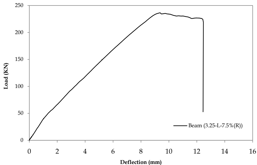
Figure 4.29: Load vs. deflection curve of FRP repaired corroded beam (series A-1)
