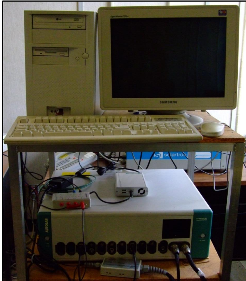
Figure 3-12. Autolab Potentiostat Model PGstat 30 used to examine ohmic and charge transfer resistances and for a measurement of hydrogen crossover current of a single PEM fuel cell.
