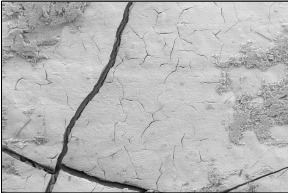
Figure 4-12. SEM surface images of (a) fresh Gore TM 57 membrane (100x magnification), (b) 100% RH cell (Run 1) with 840 hours operation (100x magnification), and (c) H 2 -air RH cycling cell (Run 2) with 622 hours operation (100x magnification).
