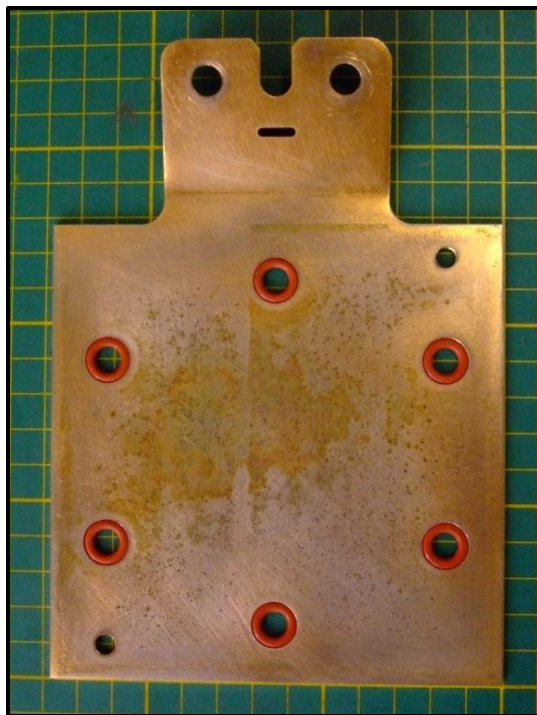
Figure A-3. An anode buss plate with six o-ring silicons.
