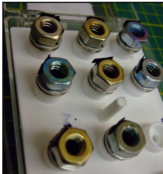
Figure 3-19. MEA samples mounted upright for SEM cross-sectional analysis.
