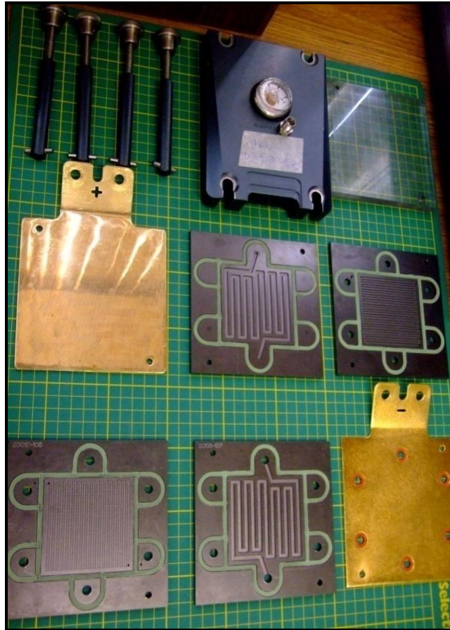
Figure A-1. Components of a single TP50 PEM fuel cell.
