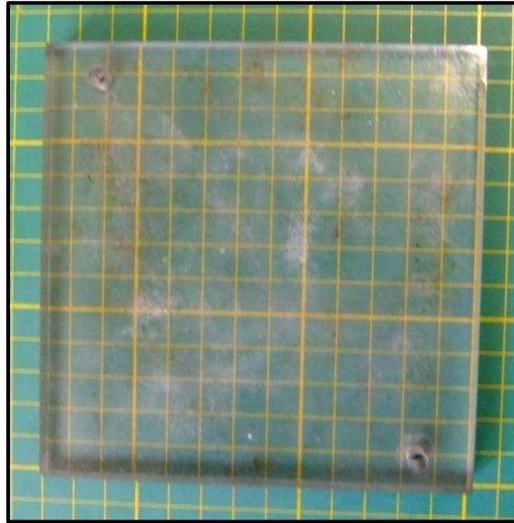
Figure 4-8. An electrical/thermal isolation plate.
