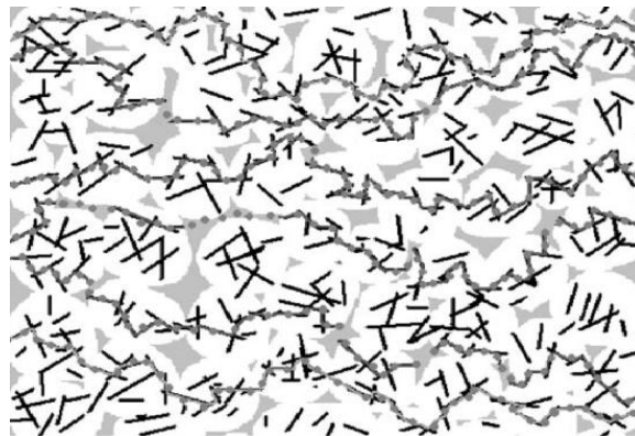
Figure 4-13: Schematic of a conductive path model [120]
