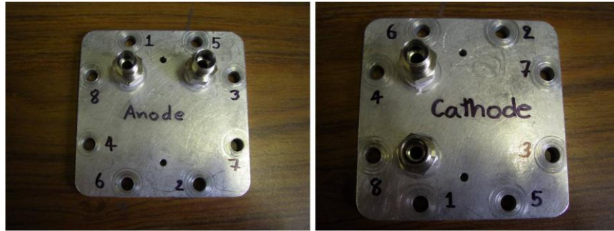
Figure B-12: An order of tightening supportive screws for fuel cell assembly
