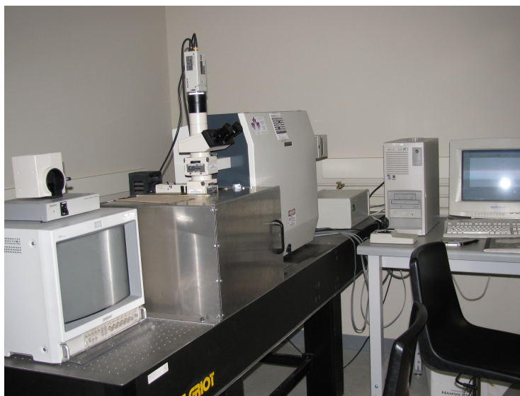
Figure 1.12: The Renishaw Raman spectrometer with a wave filter and Argon ion CW laser operating at 488 nm provided by wave filter. This laboratory is at the electrical engineering department of University of Waterloo.
