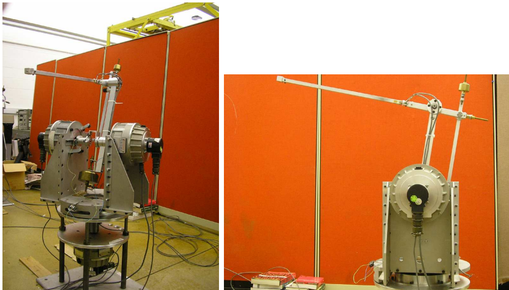
Figure 4.5: Photographs of a gravity-balanced and dynamically decoupled five-bar linkage robot at the University of Waterloo
