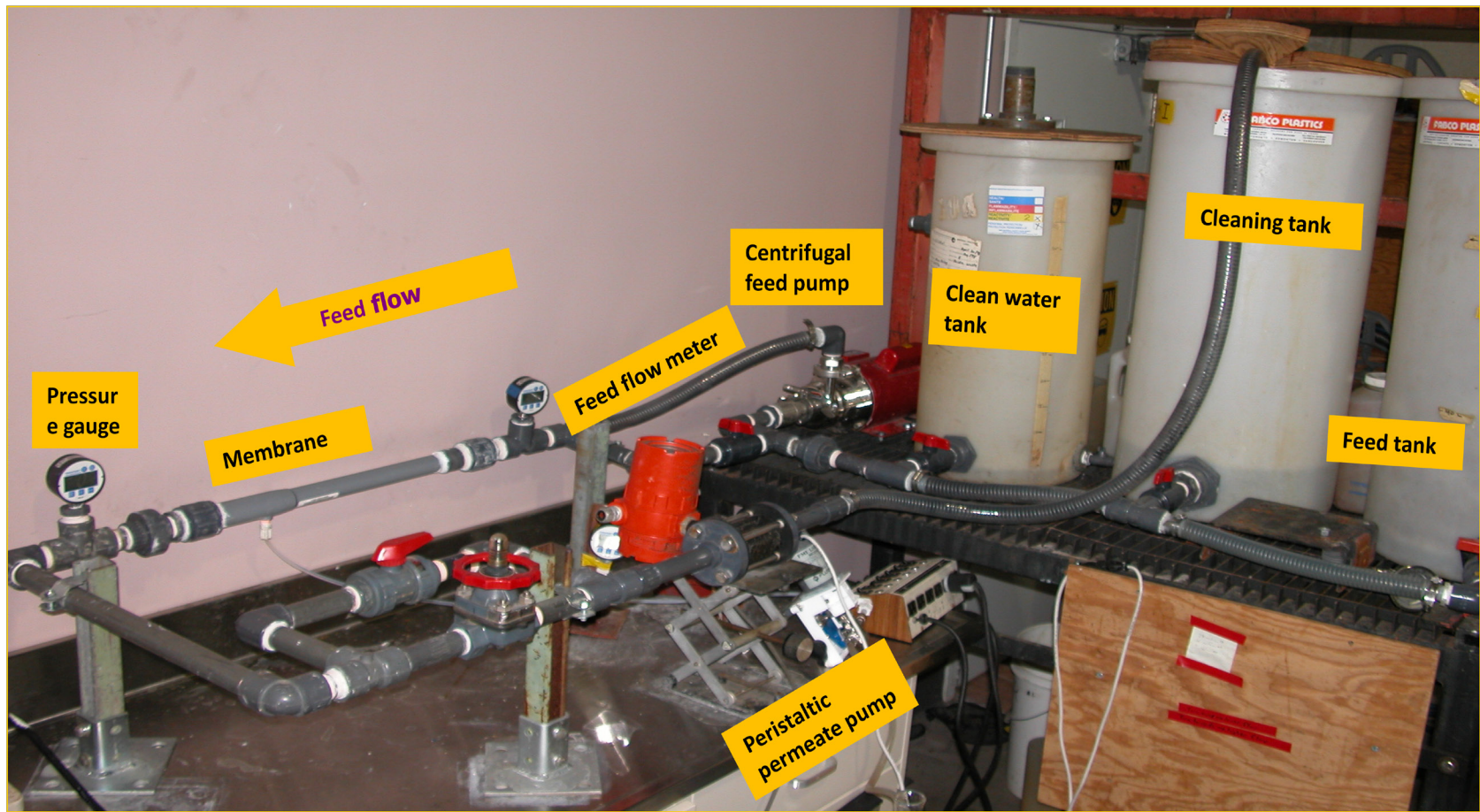
Figure A-9 Bench scale filtration unit
