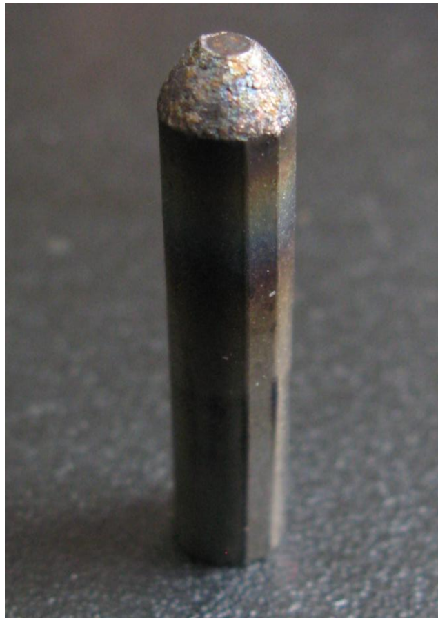
Figure 5.24: TiC p /Ni Electrode Wear with Actively Controlled Rotating and Vibrating Setup
