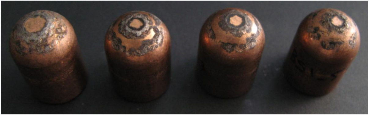
Figure 3.9: RSW Copper Electrodes Coated with Manual-Automated Hybrid Design After Partial Wearing of TiCp/Ni Electrode
