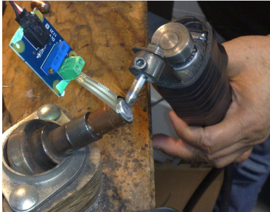
Figure 4.10: Setup for Manual Operators for Force Measurements
