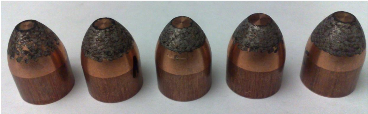
Figure 5.30: Final Coating Results with G-Code at 15 IPM
