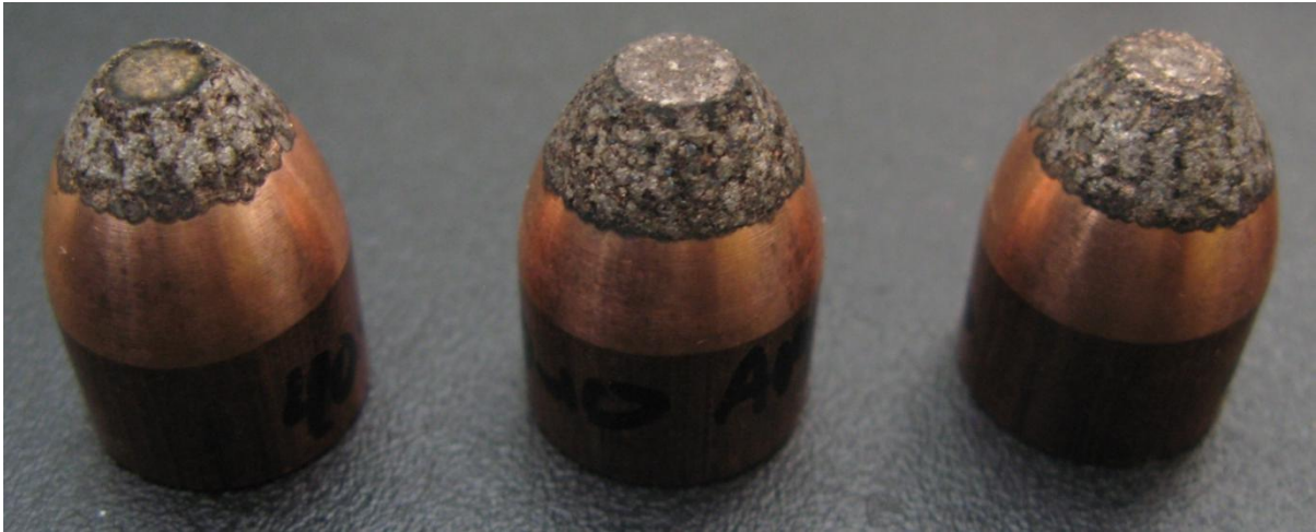
Figure 5.29: Black Deposit Throughout TiC p /Ni Coatings with G-Code Between 1 and 5 IPM
