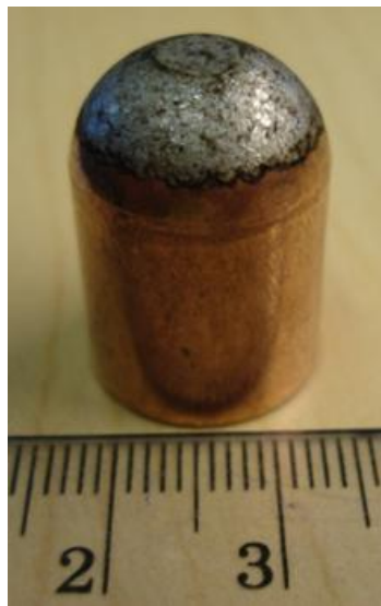
Figure 2.10: \text{TiC}_p/\text{Ni} MMC Coated RSW Cu Electrode by Manual ESD [5]
