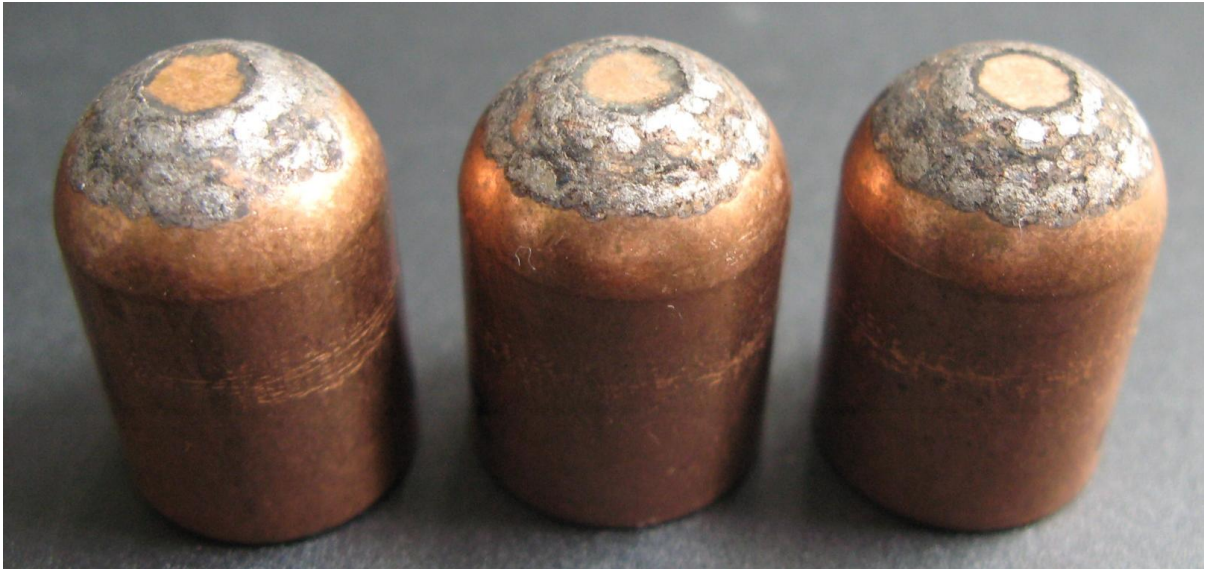
Figure 3.8: First Three RSW Electrodes Coated with Manual-Automated Hybrid Design with New \text{TiC}_p/\text{Ni} Electrode
