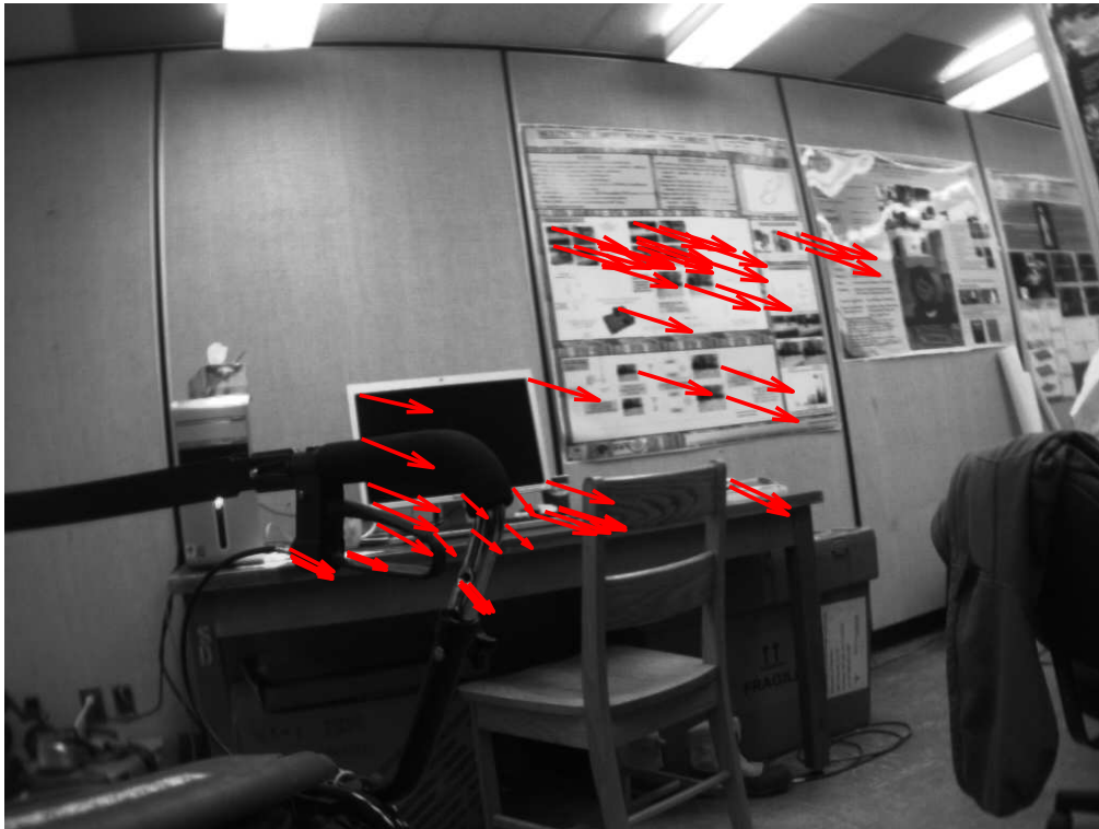
Figure 5.6: A frame from sequence 2 and the directions of the optical flow used to track the features. Mean feature displacement is 3 pixels per frame.
