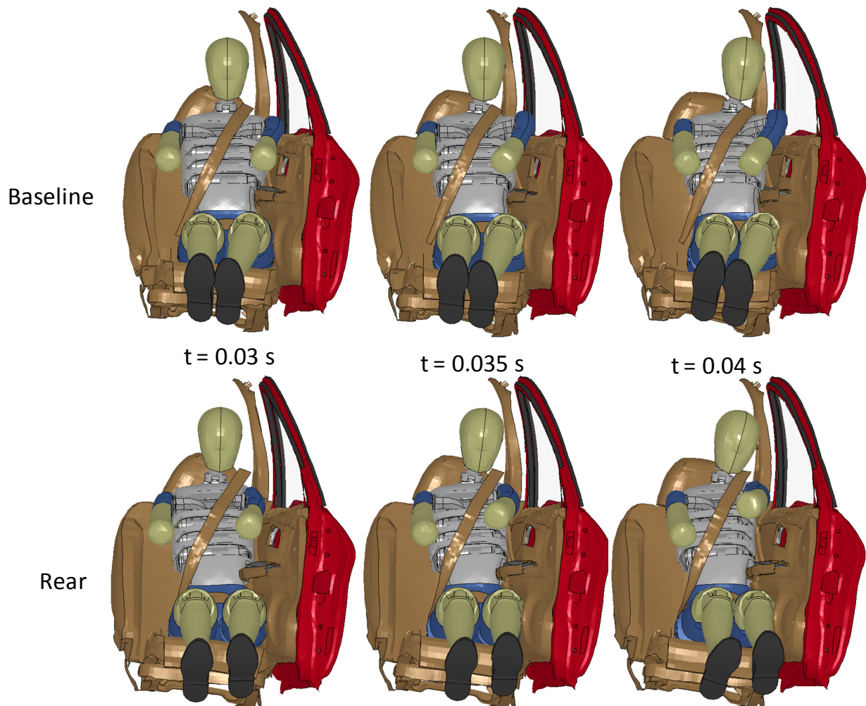
Figure 6.21: Front view of ES-2re in baseline and rear positions at NCAP barrier speed
