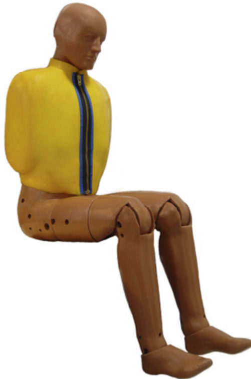
Figure 2.11: Fully assembled USSID [FTSS, 2010]
