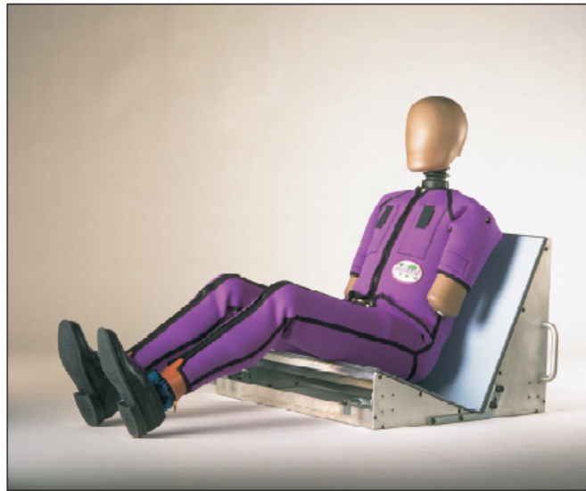
Figure 2.15: Fully assembled WorldSID [FTSS, 2007]
