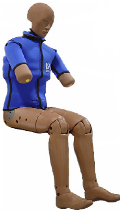
Figure 2.13: Fully assembled ES-2re [FTSS, 2005]
