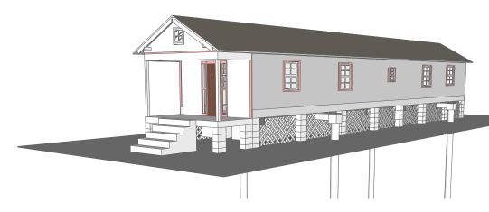
fig. 232: House on a Buoyant Foundation
