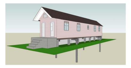
Figure 10: Rendering of a shotgun house retrofitted with buoyant foundation system.
