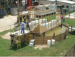
Figure 9: Full-scale testing of prototype buoyant foundation system. Constuction of prototype; stability test showing floating platform tilted due to unevenly distributed sandbags representing imbalanced live load.
