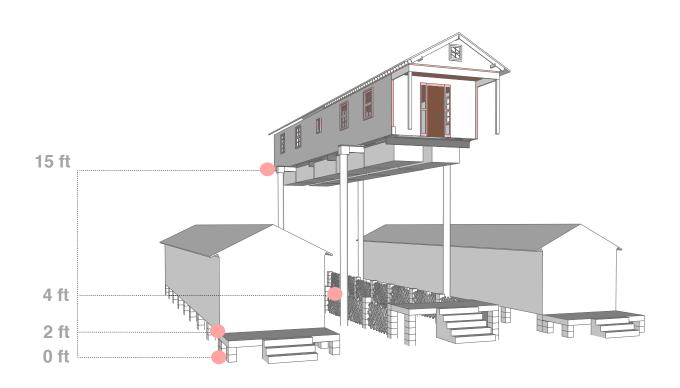
fig. 86: Shotgun House on Buoyant Foundations - Extended Position
