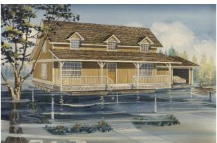
fig. 314: WLFH in 'Floating' Position
