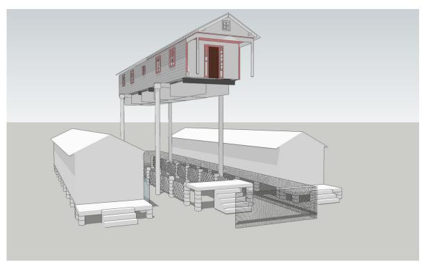
fig. 98: Conceptual Rendering of 1315 Lamanche Street Retrofit with the Buoyant Foundation System, Fully Extended
