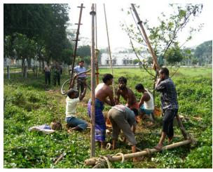
fig. 210: Digging Bore Hole for Soil Test
