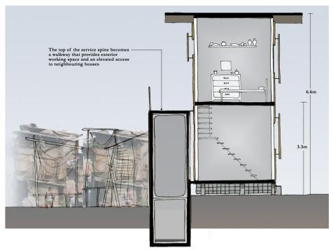
fig. 202: LIFT House, Rendered Section In Dry Conditions
