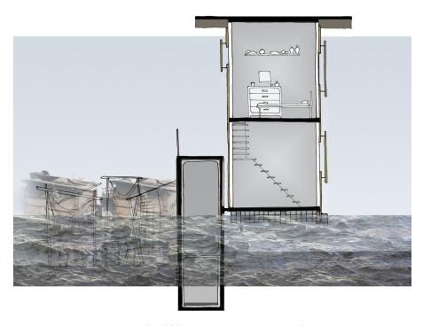
fig. 203: LIFT House, Rendered Section During a Flood
