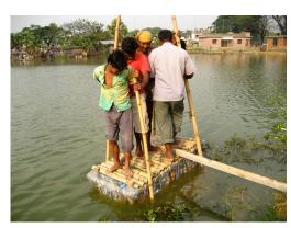
Day 11 – Sample buoyant foundation is tested with live load
