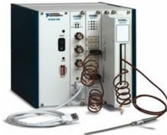
Figure 3-23 NI SCXI-1000 equipped with SCXI-1303, 32 Channel Terminal.
