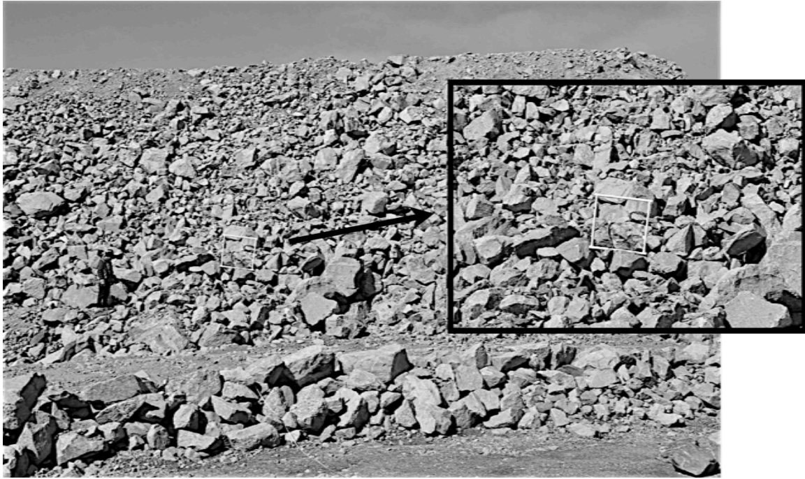
Figure 2 - 4: A typical face of the piles with 1m x 1m PVC reference square.
