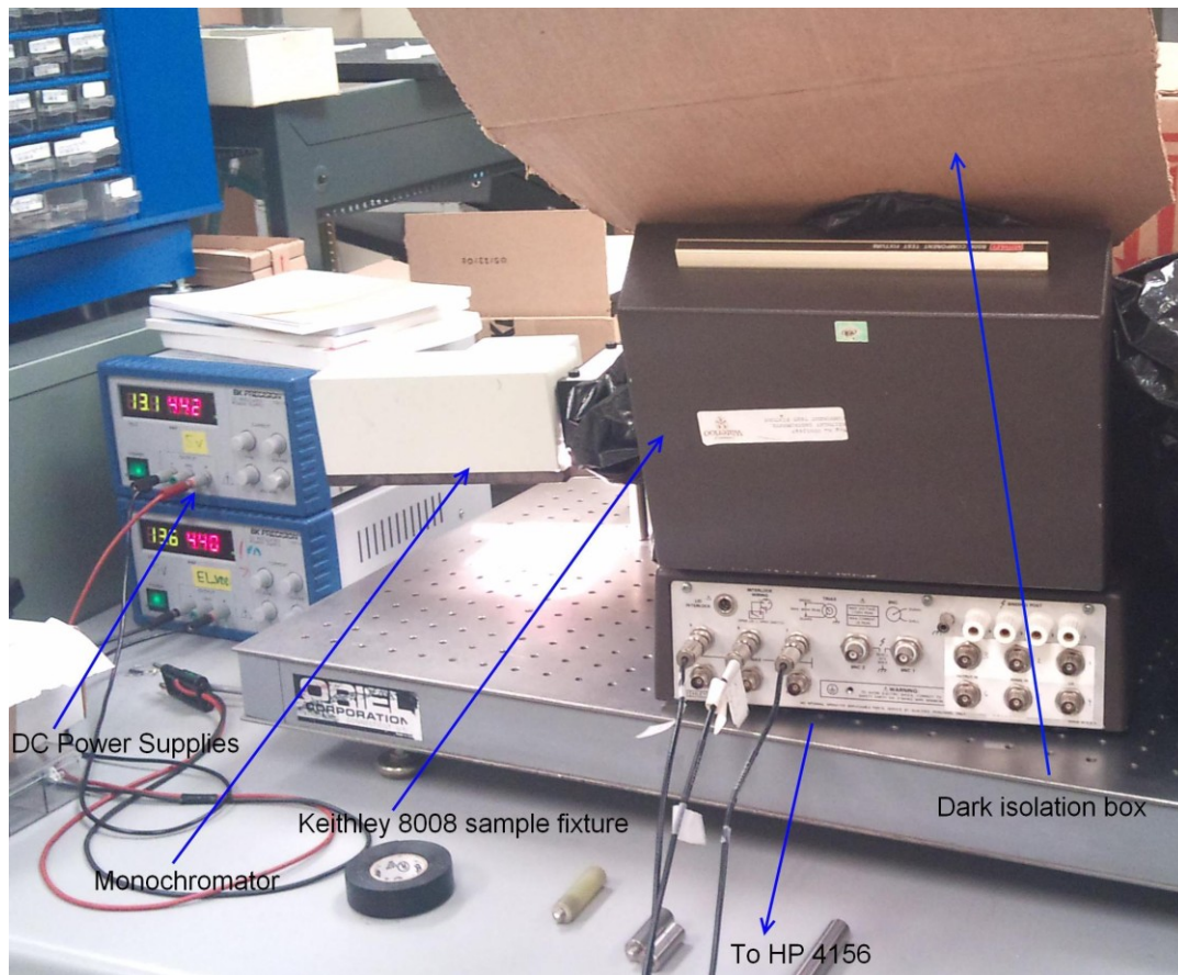
Figure 43 : EQE Setup
