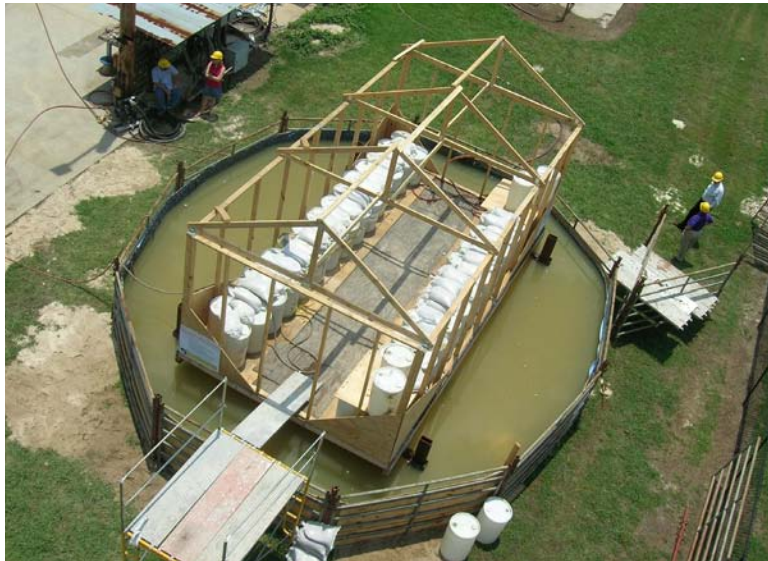
5.11. LSU prototype demonstrating floatation of amphibious structure
