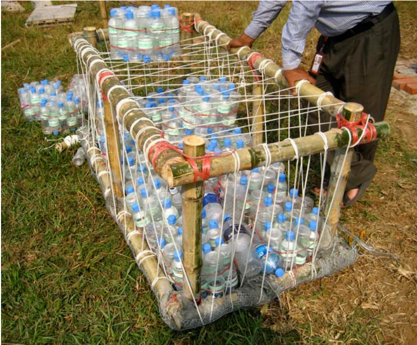
8.35. Water bottle foundation model
