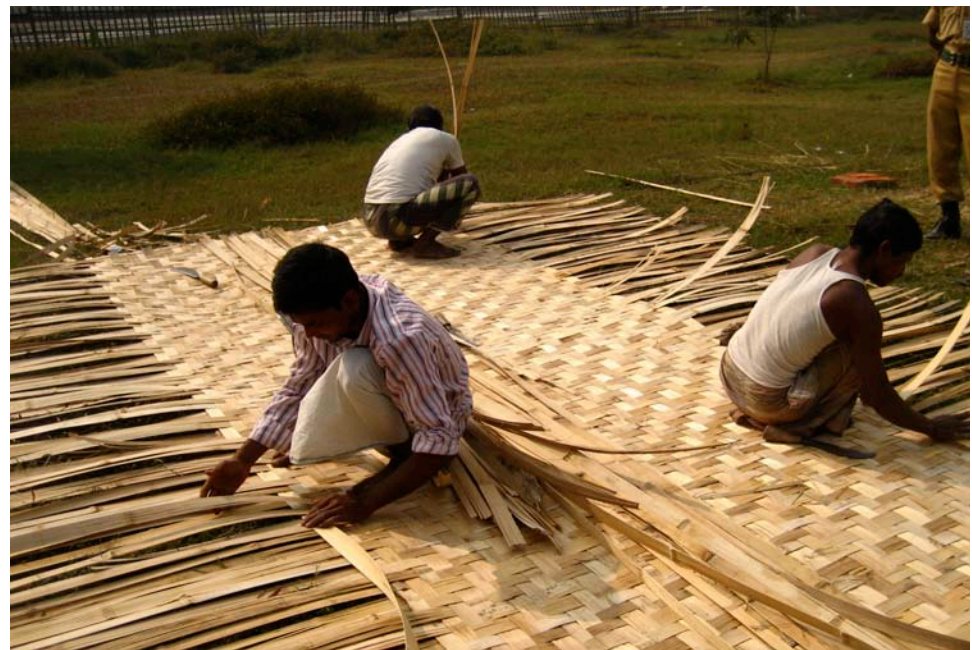
8.95. Bamboo mats woven for interior walls
