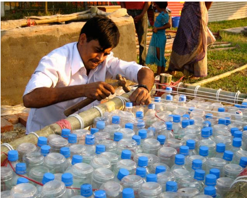
8.36. Volunteer attaching ropes to encase the used water bottles in preparation for testing
