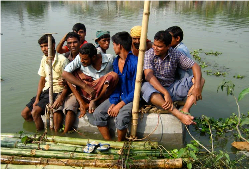
8.42. Live load test showed greater capacity than the water bottle foundation in similar size
