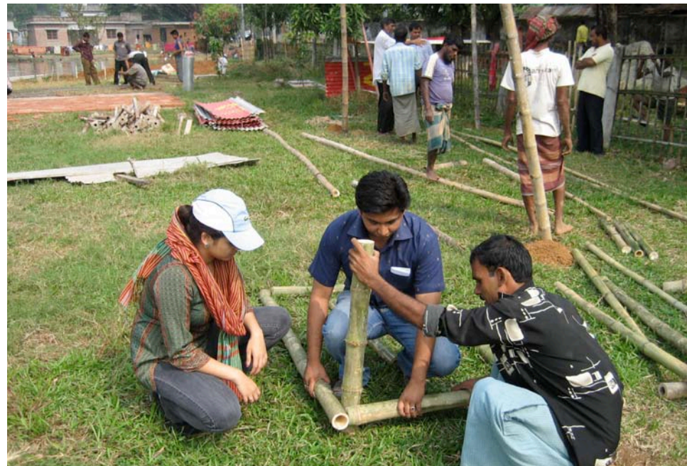
8.34. The start of the foundation models for testing
