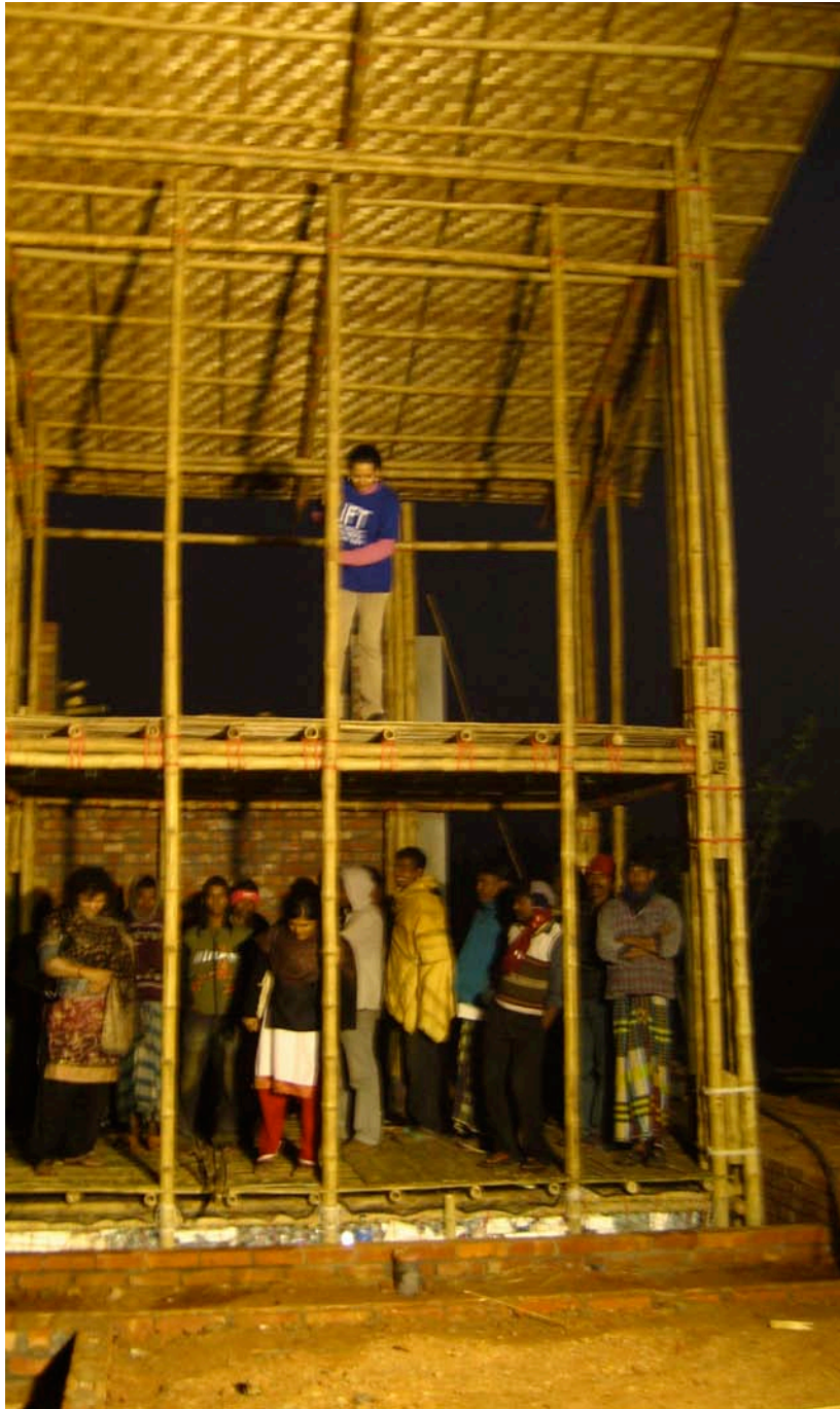
8.112. Buoyant dwelling tested with live load
