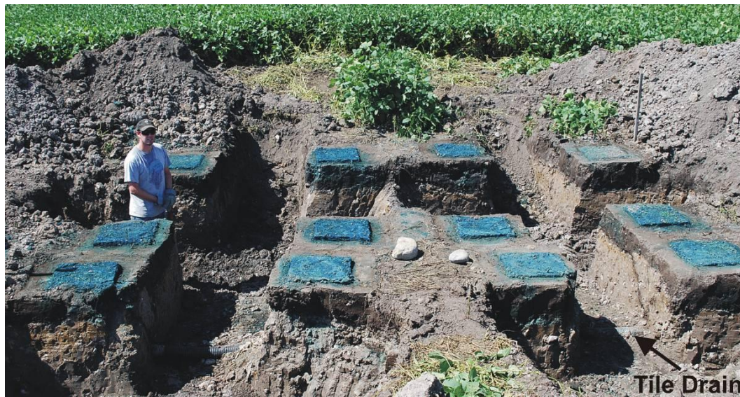
Figure 2.3. Photograph showing plot 1 after the infiltration tests, dye application and trenching had been conducted.
