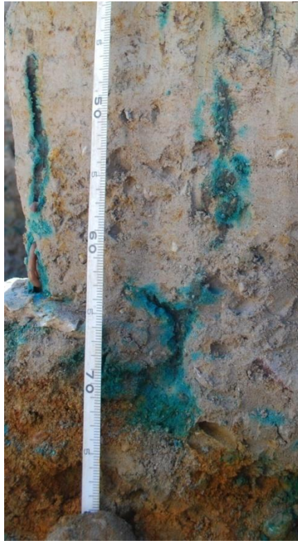
Figure 2.6. Photograph taken at plot 3 that shows the typically vertical orientation of the worm burrows in the B horizon, and how the macropores terminated as the soil composition transitioned to coarser material.
