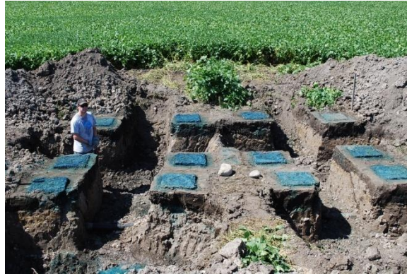
e) Macropore counting surface preparation
