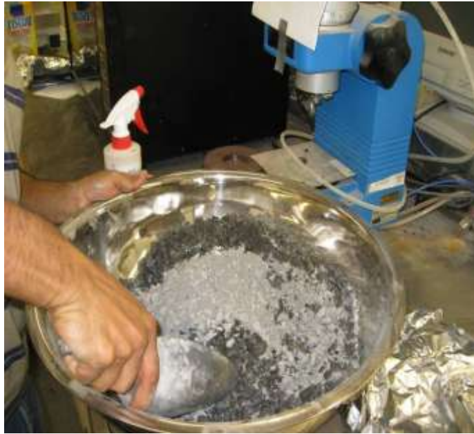
Figure 3-8 : Mixing of Aggregates with Additives
