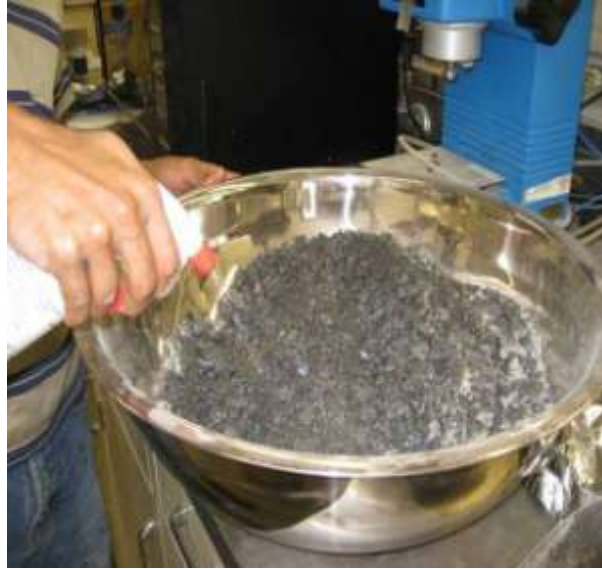
Figure 3-6: Application of UP5000 to Aggregates
