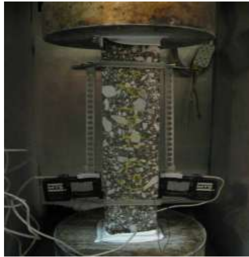
Figure 4-16: TSRST Instrumentation in the Environmental Chamber and MTS-810
