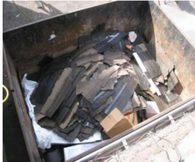
Figure 2-2 : Tear-off Shingles after Service Life
