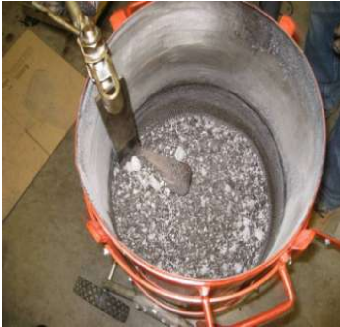
Figure 3-10 : Mixing of Aggregates and AC
