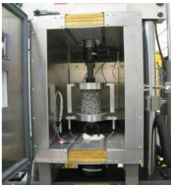
Figure 4-4 : A Test Specimen in the Environmental Chamber for Dynamic Modulus Test
