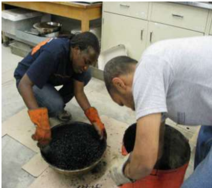
Figure 3-11 : Mixing of Aggregates and AC
