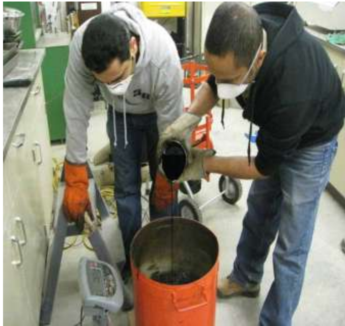
Figure 3-9 : Addition of AC to Aggregates
