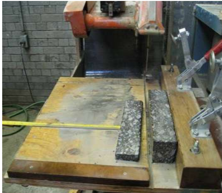
Figure 4-12: Saw Cutting of Fatigue Beams
