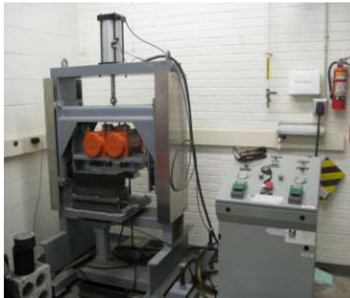
Figure 3-2 : CPATT Asphalt Vibratory Compactor (AVC)
