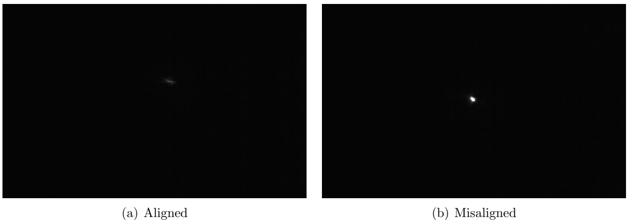
Figure 4.8: Images from the tilt alignment monitoring camera. Shown is a view of the system properly aligned as well as a view of the system severely misaligned.
