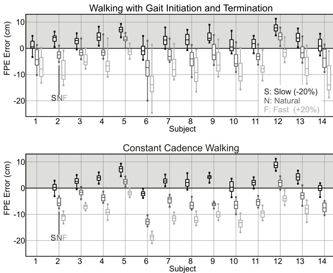
Figure 6.4: Box and whisker plots of the error between the FPE and each subject's lateral malleolus at foot contact. Whiskers run between the 5 th and 95 th percentiles, boxes between the 25 th and 75 th percentiles with a hash at the 50 th percentile. Natural paced trials align with the subject number; slow trials are immediately to the left and fast trials are to the right. Subjects are motivated by not only balance but pace and acceleration since they step further behind the FPE as they walk faster, and with more variation when they initiate and terminate gait. I failed to collect constant cadence trials for subject 1
