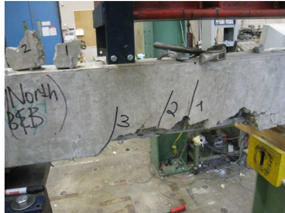
b-Beam after complete failure
