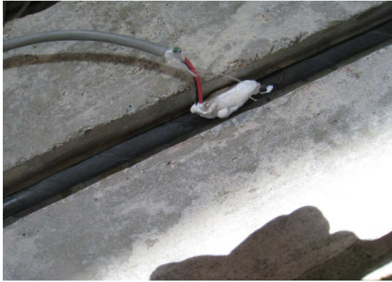
a- Strain gauge on CFRP rod
