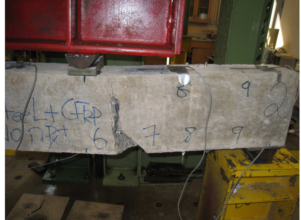
b-The same crack after complete failure with chunk of concrete separated
