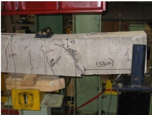
a-Major crack in shear span after failure
