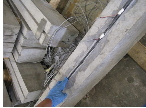
b- Rod placed and pressed into the epoxy
