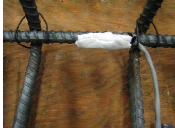
b- Strain gauge on steel rebar
