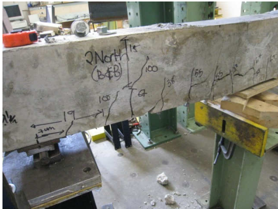
a-Cracking in shear span before chunk separation
