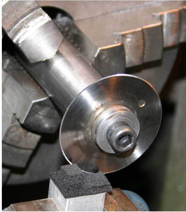
Figure 3.1: Preparation of the foamed specimen for micrographic analysis.
