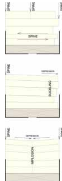
Figure 2.33. Diagram showing implications with placement of books, where the top image is the ideal method.
