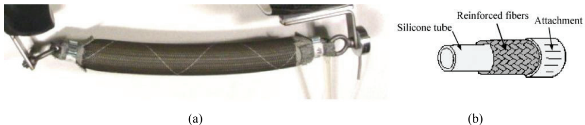
Figure 2.6: McKibben air muscle (a) in situ in an orthosis (adapted from [56]) and (b) detailing air muscle constitution (from [62]).
