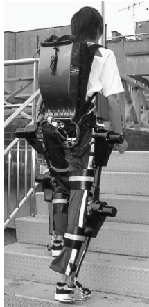
Figure 2.16: Hybrid Assistive Limb 3, HAL-3 (from [87]).
