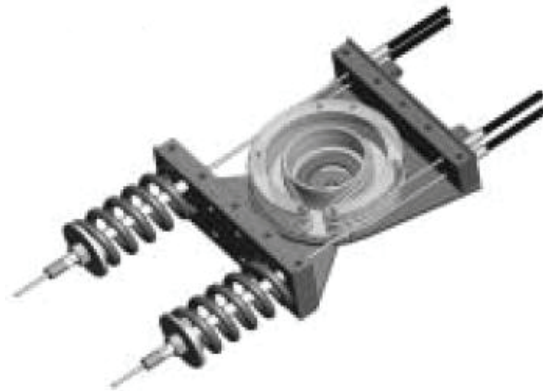
Figure 2.30: Bowden cable actuator for the LOPES rehabilitation orthosis (from [104]).
