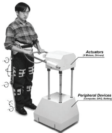
Figure 2.28: Portable bilateral walking assist orthosis for the elderly (from [103]).
