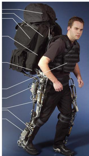
Figure 2.14: The Berkeley Lower Extremity Exoskeleton, BLEEX (modified from [73]).
