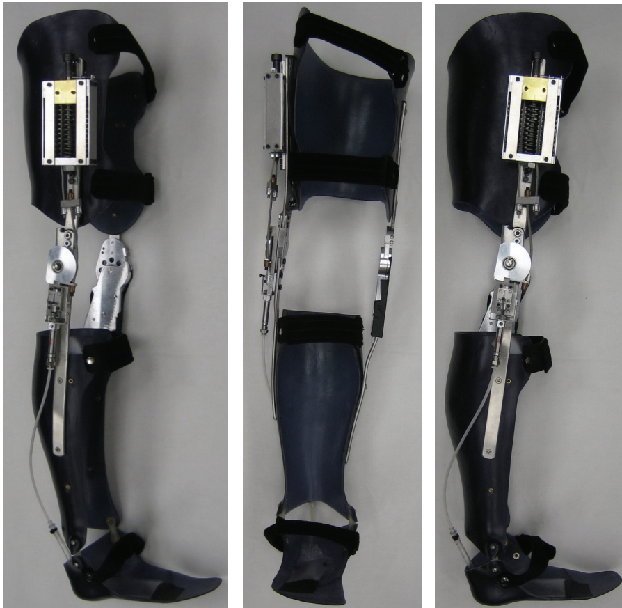
Figure 5.1: KEA prototype mounted on a preexisting right-leg KAFO for biomechanical trials.
