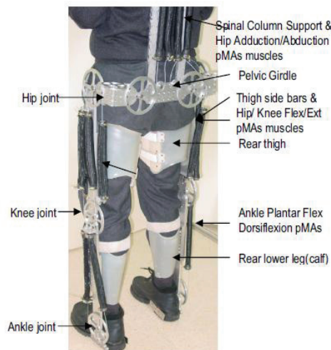
Figure 2.34: Ten degree-of-freedom lower-body orthosis. Actuated by antagonistic PMA pairs (from [58]).
