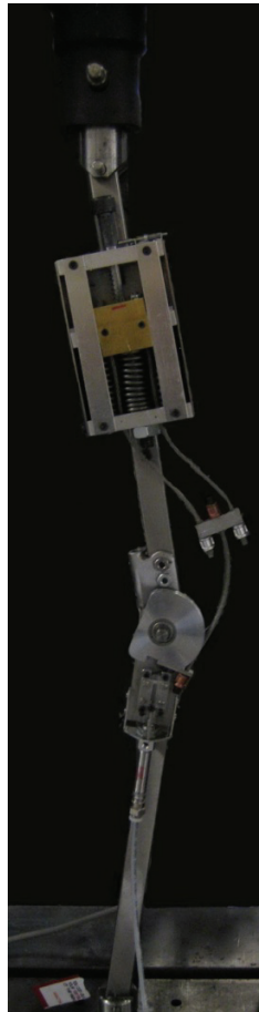
Figure 4.11: Photograph of the KEA during the function tests after undergoing extension with the springs locked in a compressed state. The knee disk is automatically unlocked by the actuator return spring when extension occurs with the springs locked in a compressed state.
