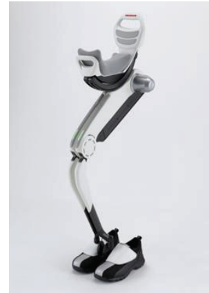
Figure 2.17: Honda's walking assist device with bodyweight support system (from [77]).
