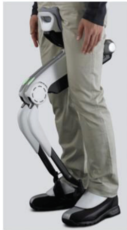
Figure 2.19: Honda's walking assist device with bodyweight support system (from [77]).
