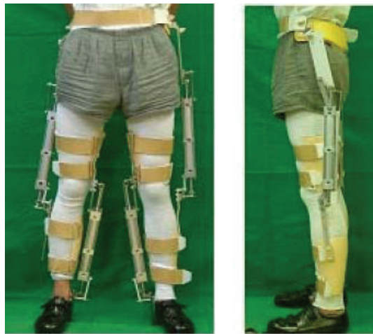
Figure 2.36: Biarticular hydraulic actuator placement (from [51]).
