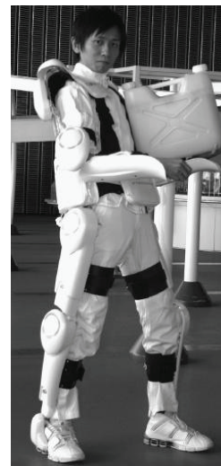
Figure 2.15: Full body exoskeleton, Hybrid Assistive Limb 5, HAL-5 (from [87]).
