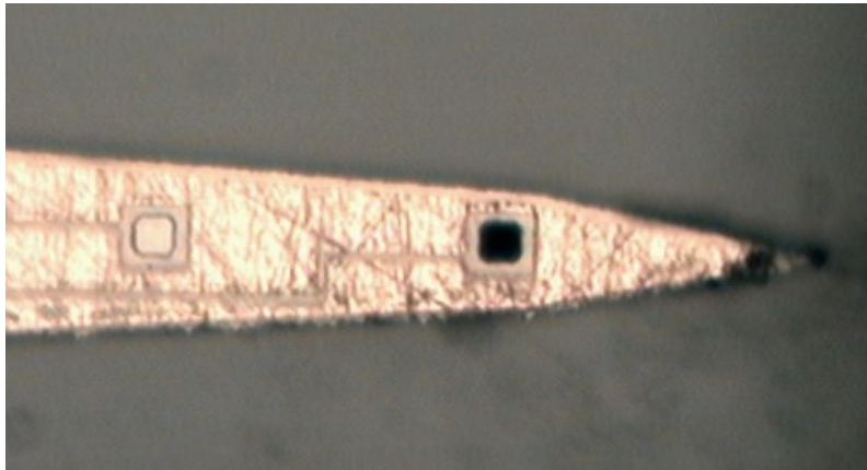
Fig. 3.16: The optical images of an electrode site after the pulse test.
